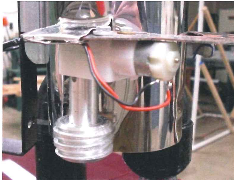
Figure 2: Cup Dispenser Motor with Cup Screw
