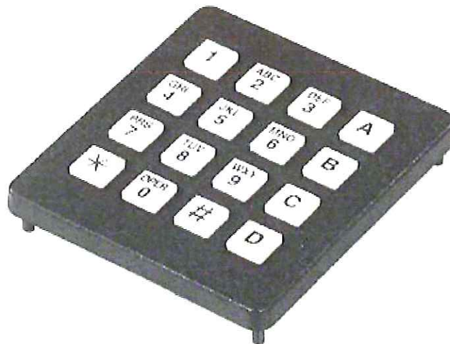
Figure 14: 4x4 Matrix Keypad
