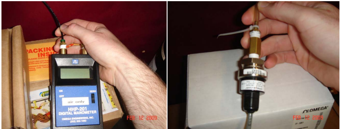
Figure 6. Hose connections to PT and digital manometer
