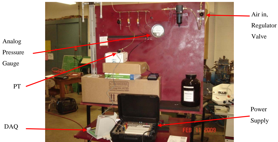
Figure 5. Level meter testing configuration
