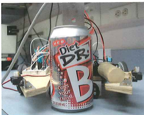
Figure 20: Can in position to be picked up
