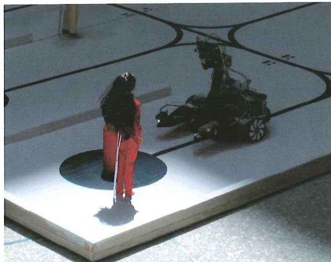
Figure 23: The Falcon failing to detect the red can
