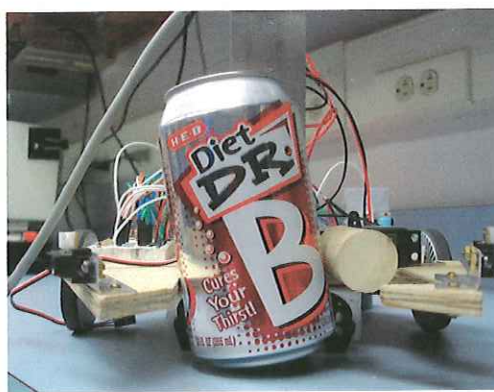
Figure 21: Can manipulator gripping soda can
