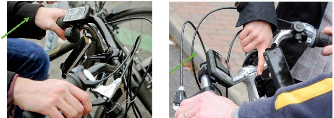
Figure 4. The handle-bar mounted panel for switching the assistance on/off and selecting the level of assistance (low, medium, high), for the the Raleigh Dover (left) and the Velo-cité (right) model.
