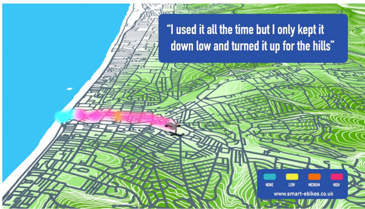
Figure 8. Visualisation of a user trip where the assistance was increased when going uphill, with quote by the same user.
