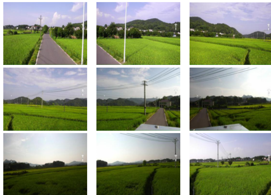
Figure 34. Images captured by the experimental vehicle. The FoV of the camera is 50^\circ and each image was captured every 40^\circ rotation of the camera. The resolution of each image is 1920 \times 1080 . It can be seen that there are some overlaps between the adjacent images.
