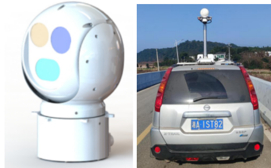
Figure 33. Equipment used in the experiment: (Left) Camera can be rotated and images are captured by command; and (Right) installation of the camera on the experimental vehicle.
