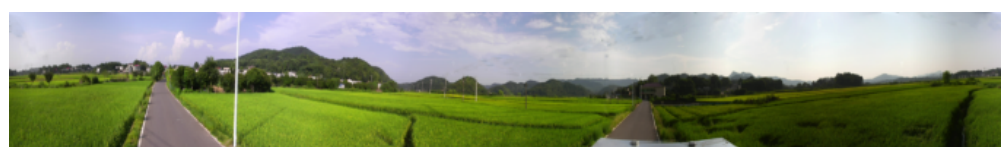
Figure 35. The panoramic image. Using the image stitch algorithm, the sub images in Figure 34 are merged into a panorama. The left side is the image captured when the optical axis of the camera coincides with the central axis of the vehicle.
