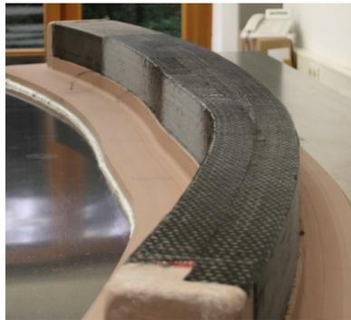
Figure B.9: The preform made from non crimp fabric.
