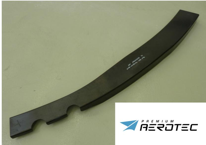
Figure B.5: The composite test frame studied.
