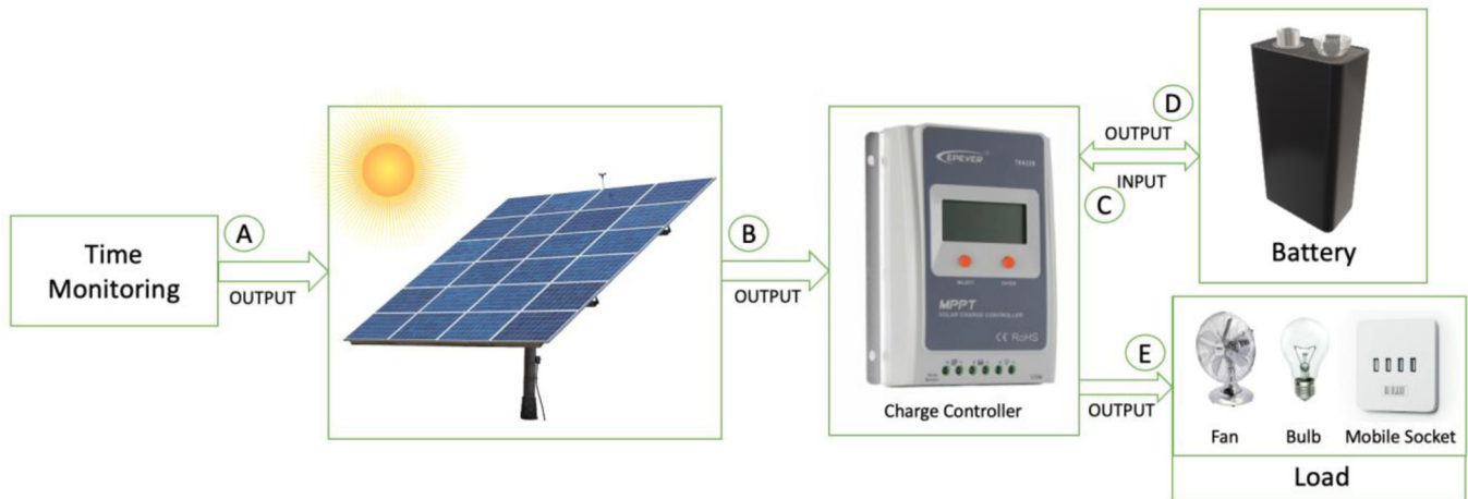
Fig. 1. The flow of energy diagram for the household installed at Odisha, India.
