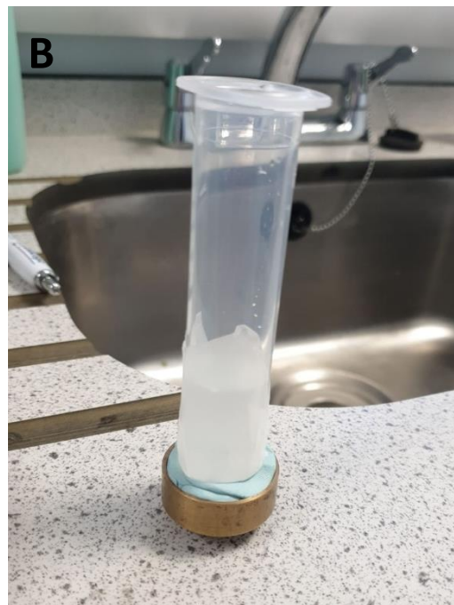
Figure 3.4- Mounting system for a porcine corneoscleral disc for microCT.
