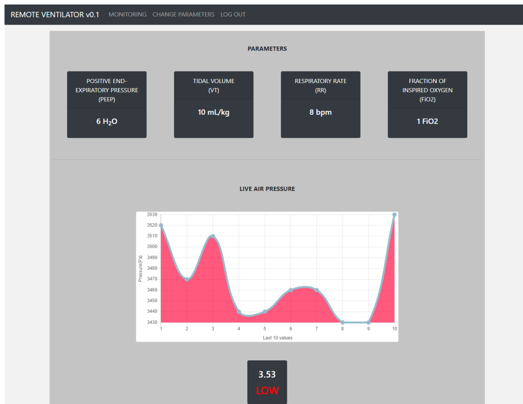
Figure 9. Remote ventilator dashboard reflecting the change in parameters over the communication network.
