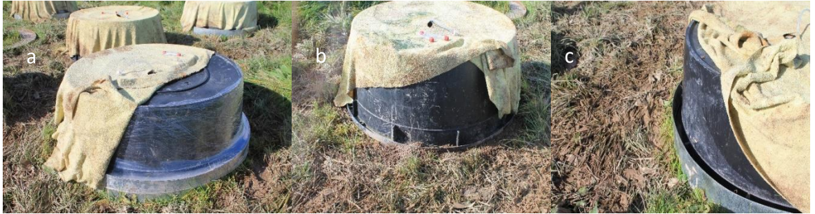
Figure A1. a) Chamber seal with metal ring and plastic wrap, b) chamber without ring, and c) chamber with metal ring.
