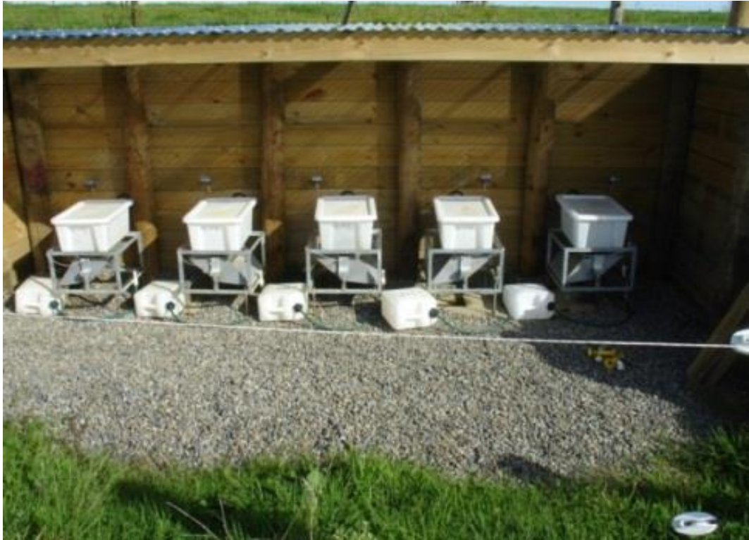
Figure 3.2. Individual tipping buckets for collection of drainage water in one of the collection shelters.
