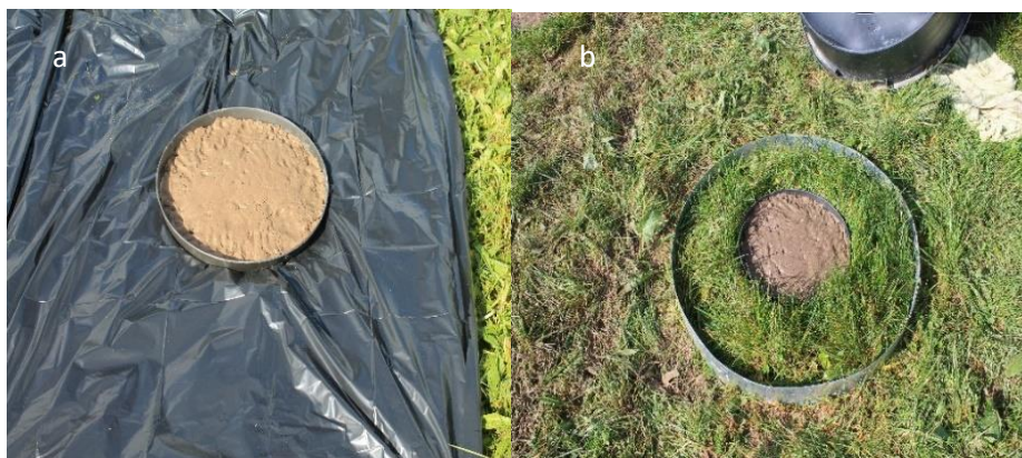
Figure A2. a) Chamber's floor is cover with a plastic bag; b) chamber's floor is uncovered. These chambers were sealed with a bicycle tubes, which were inflated to provide a gas-tight seal.
