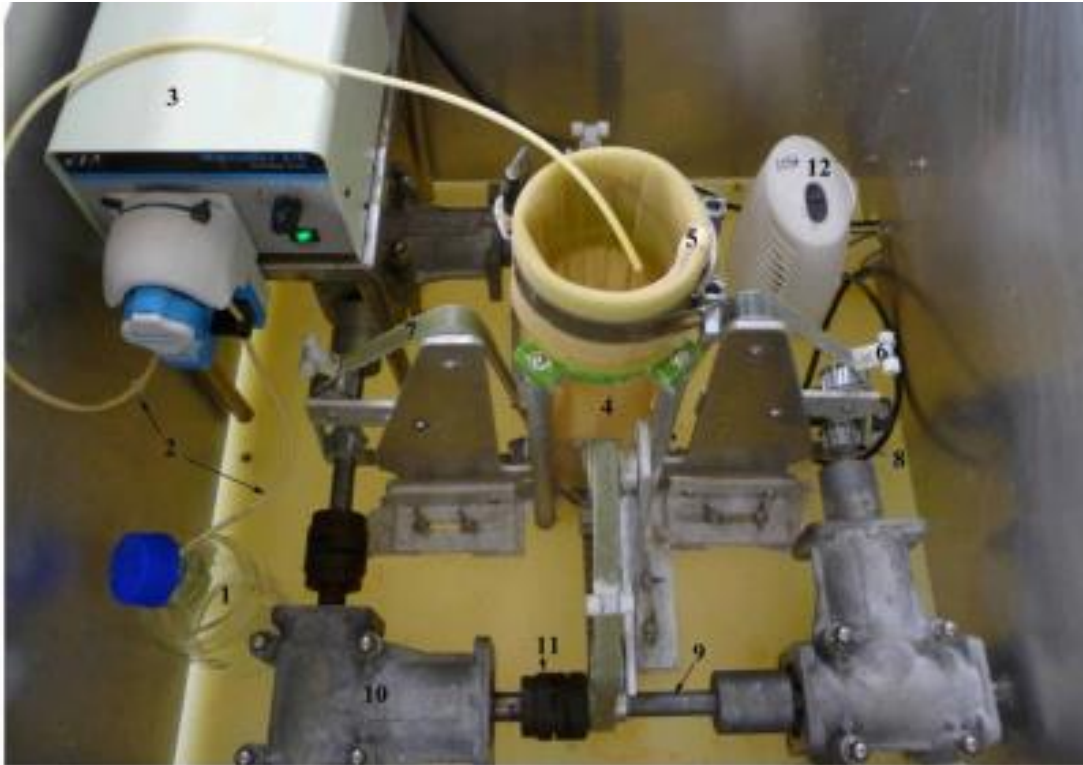
Figure 3-3 The human gastric simulator and the latex stomach chamber. 1: SGF; 2: plastic tubes for secretion; 3: pump; 4: latex gastric chamber; 5: mesh bag; 6: roller; 7: belt; 8: pulley; 9: shaft; 10: angle gear; 11: Love-Joy joint; 12: fan heater for temperature control (Ye, Cui, Dalglish, & Singh, 2016)
