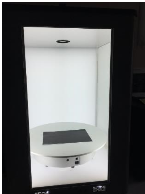
Fig. 6-5: Petri dishes containing the boluses were placed inside ScanCube 308 which conferred a standardised brightness. A camera is used to capture the image of the bolus.
