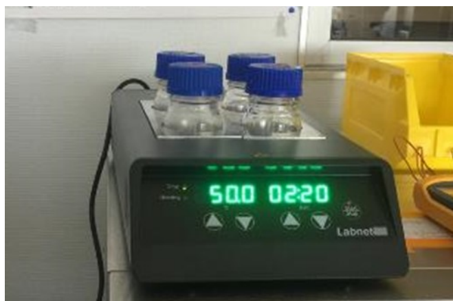
Fig. 6-10: Rice samples in Schott Vials placed inside warmer that was set at 50°C.
