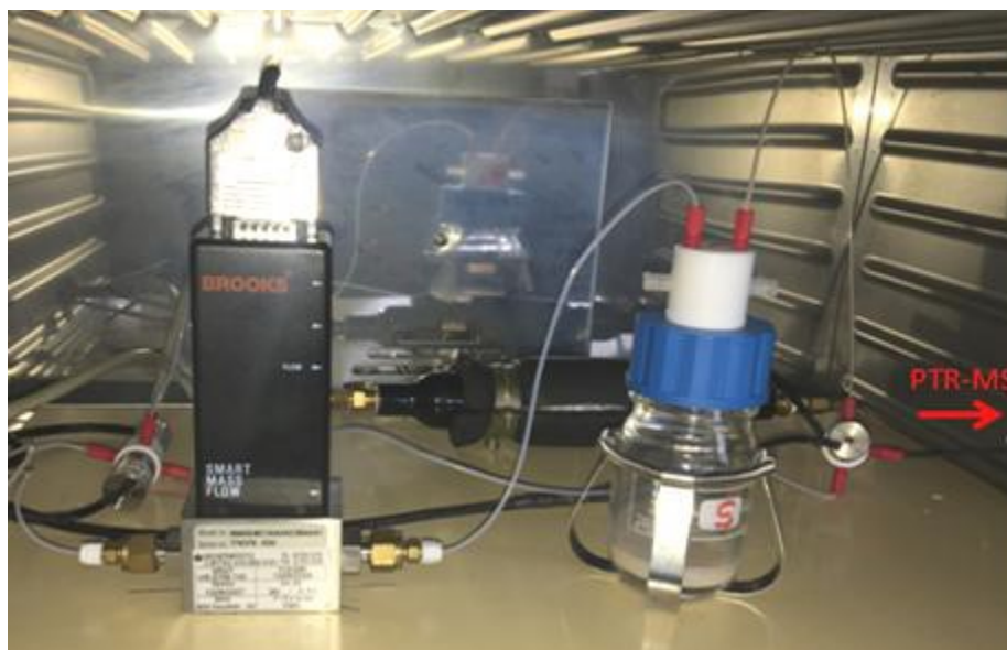
Fig. 6-8: In vitro set up to measure aroma compounds in rice using the PTR-MS
