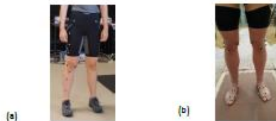
Figure 1: Example of reflective markers placed while wearing shoes (a) and barefoot (b)
