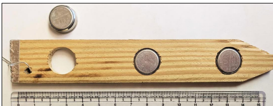
Figure 1. A complete iButton stake that will measure soil depths 5, 10, and 15 cm when installed with the top of the stake (picture left) 2 cm below the soil surface.
