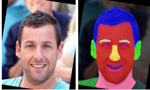
Figure 4.2: Visualization of a segmentation mask output by the DeepLab v3+ network.
