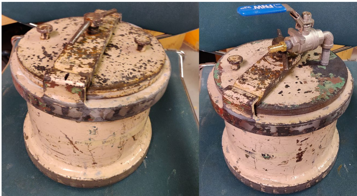
Fig 3. Regular Mill Lid (left) and Tapped Mill Lid with Valve (Right)
