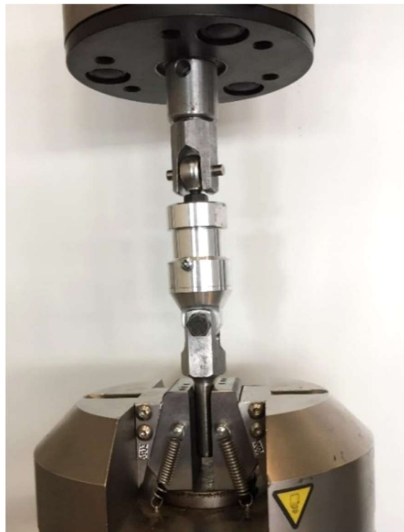
Figure 5.5 Test setup of the STF damper in a dynamic test instrument.
