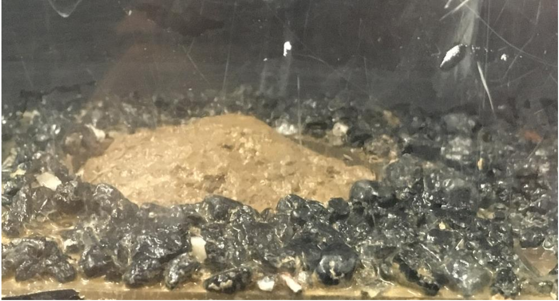
Figure 4.22 Example of Cone shaped erosion pattern
