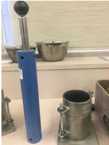
Figure 3.3 Rammer (left) and mold (right) used to compact soil
