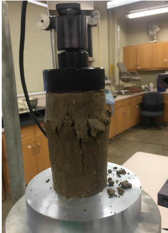
Figure 3.12 Soil Specimen after failure
