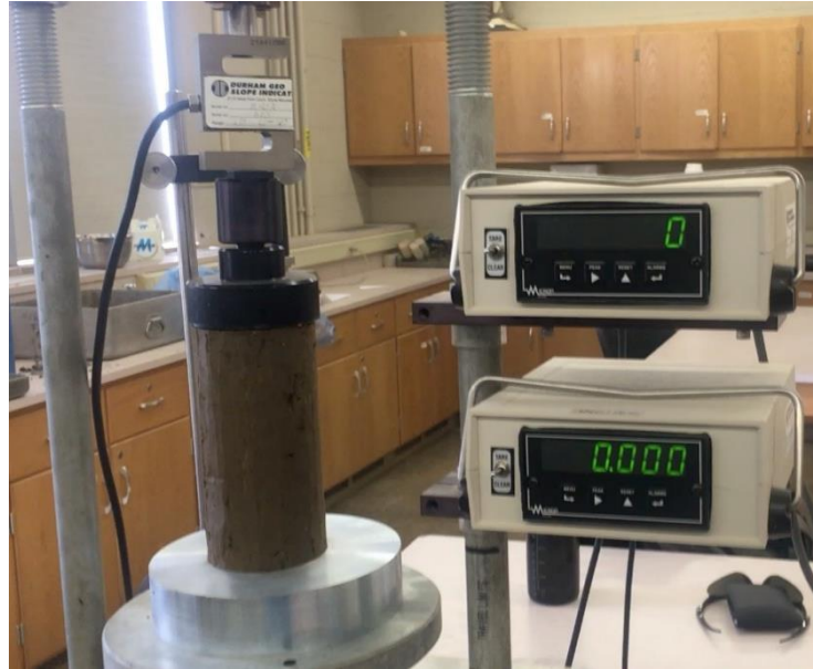
Figure 3.10 Specimen tested for Unconfined Compressive Strength
