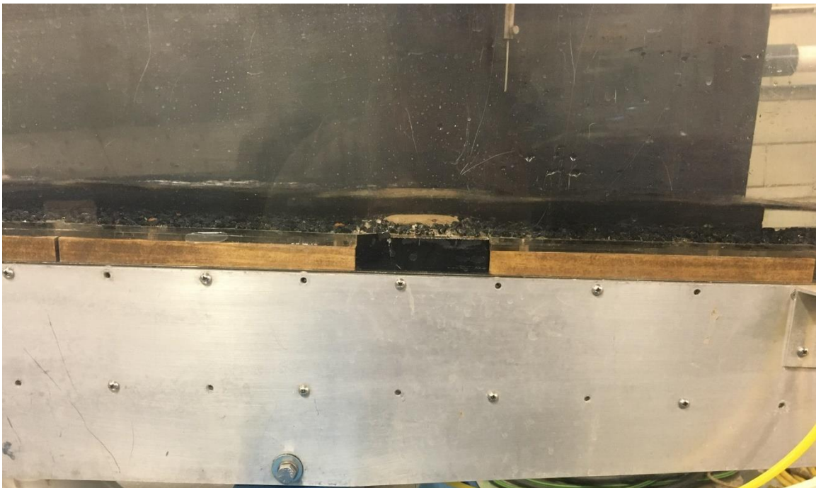
Figure 4.2 Soil sample at start of erosion test
