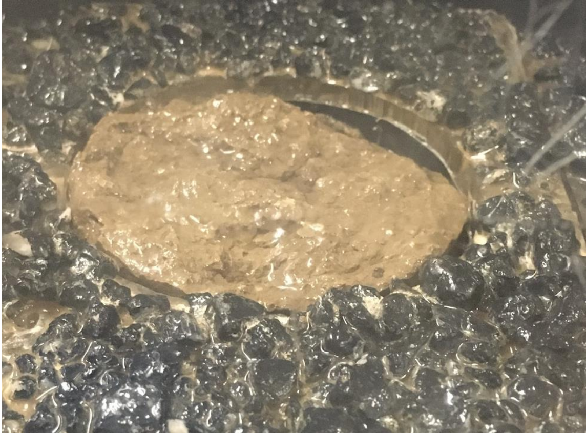
Figure 4.19 Final erosion depth after about 5-hours
