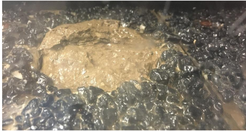
Figure 4.3 Soil sample after erosion test is complete
