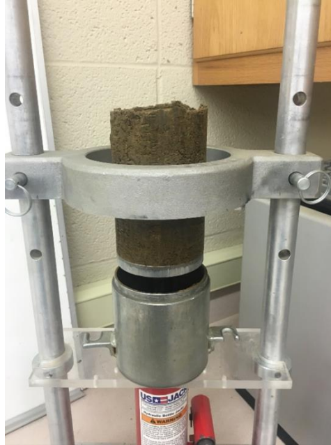
Figure 3.7 Specimen being extracted from Proctor Mold
