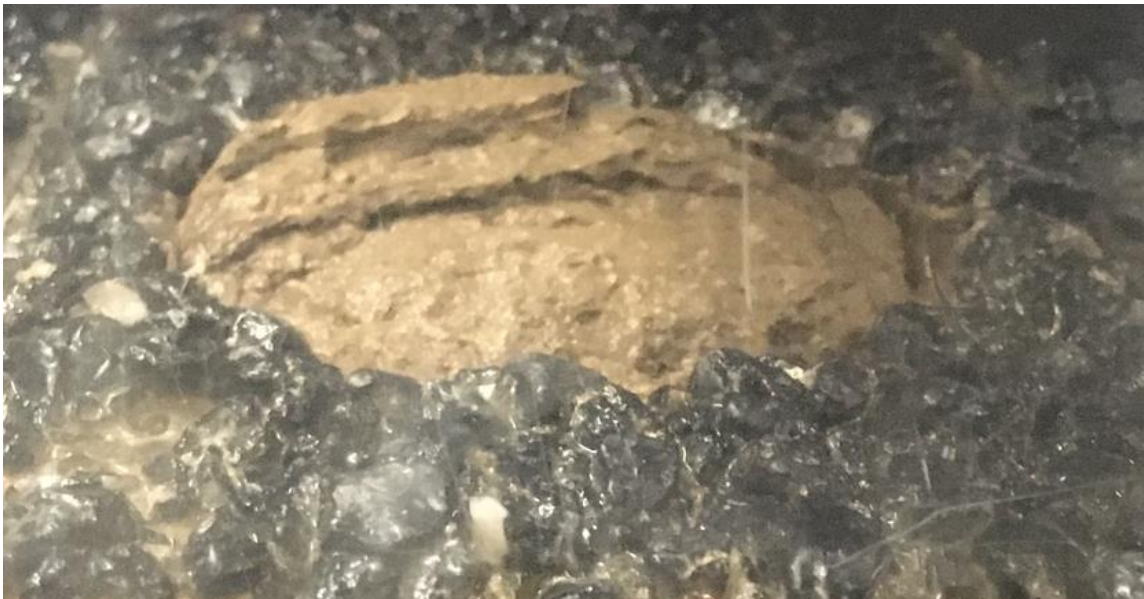
Figure 4.21 Example of block erosion pattern from side-to-side
