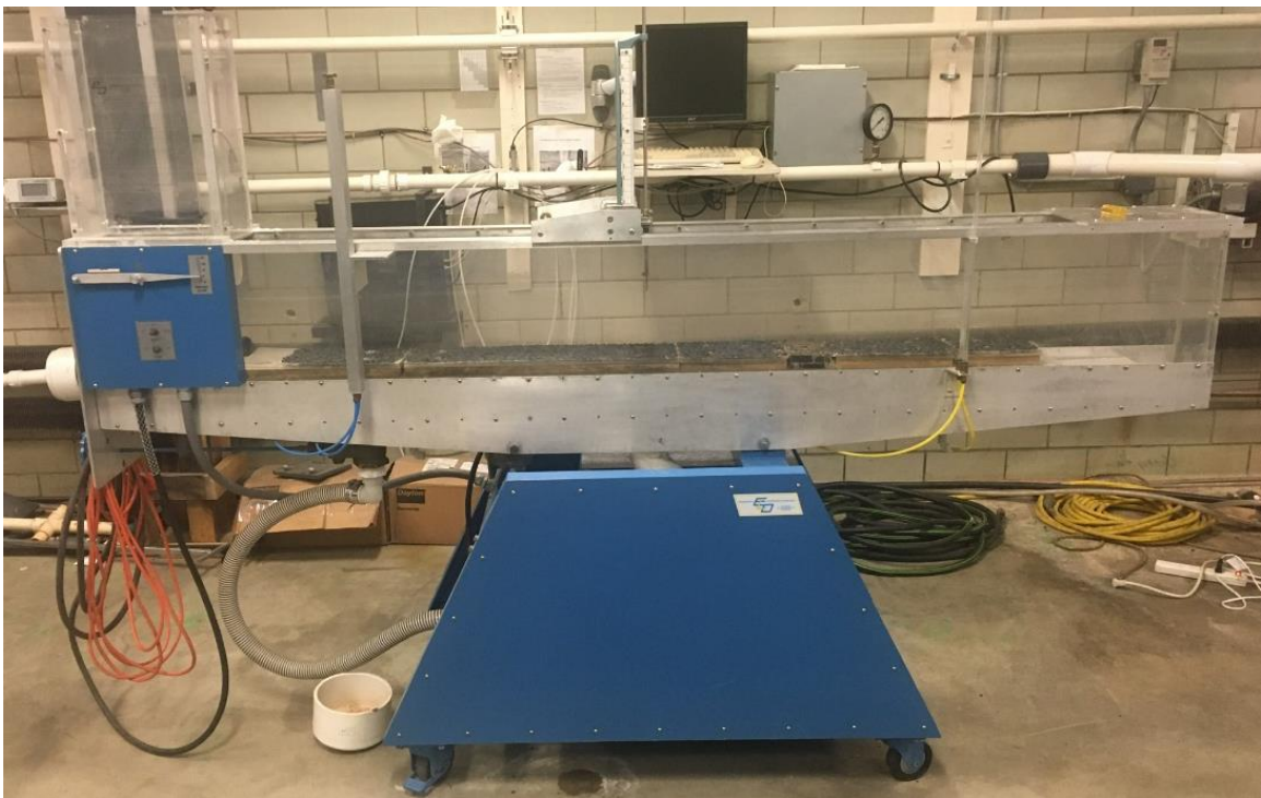
Figure A.1 A-8 Hydraulic Channel
