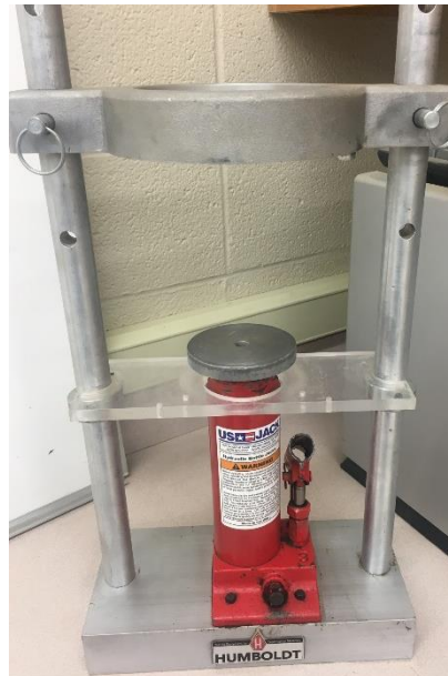
Figure 3.6 Jack used to extract specimen from Proctor Mold
