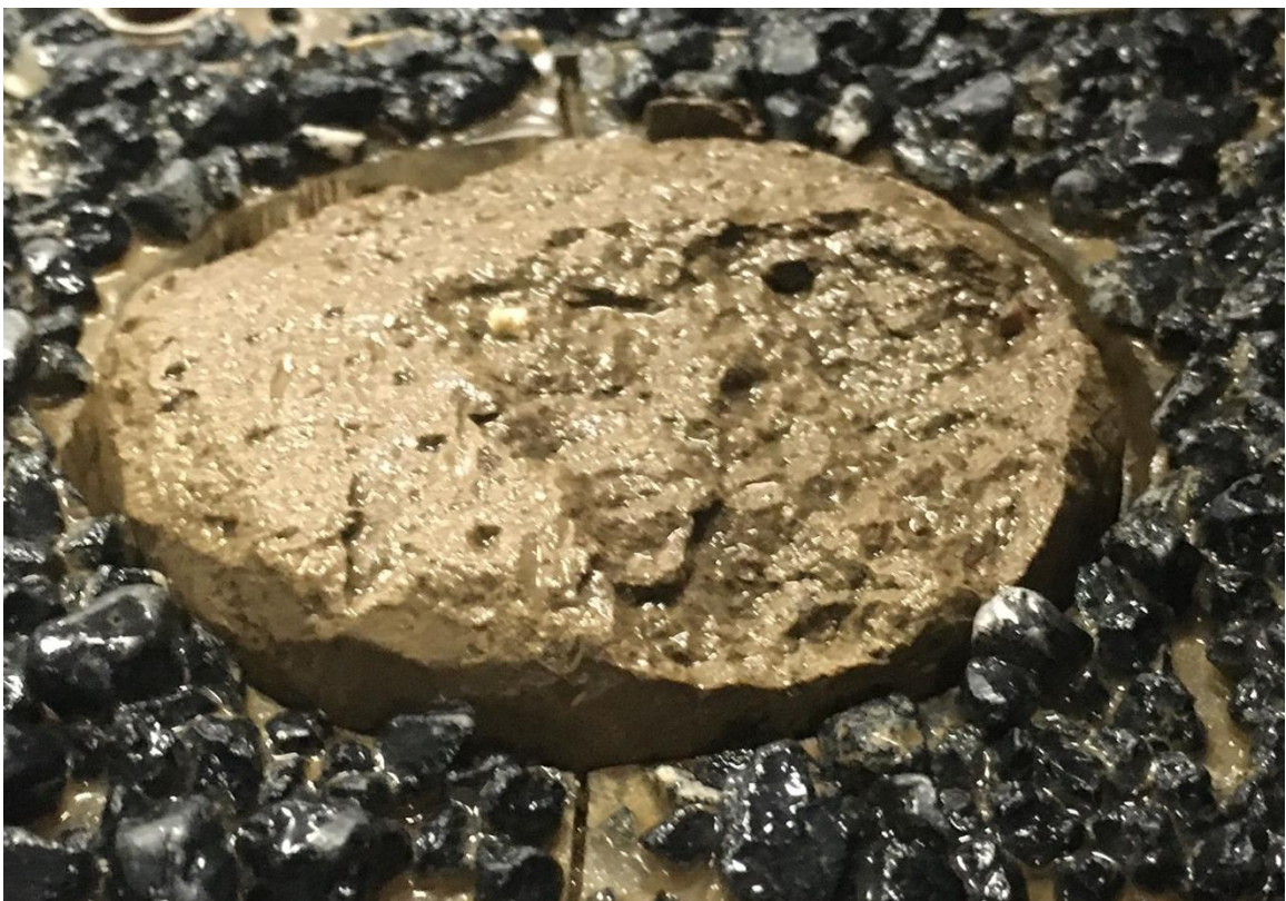
Figure 4.23 Example of a non-uniform erosion pattern in the downstream portion of soil sample
