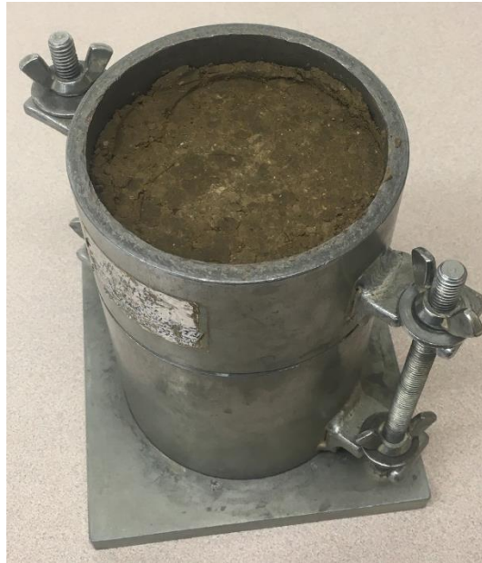
Figure 3.5 Specimen after full compaction effort
