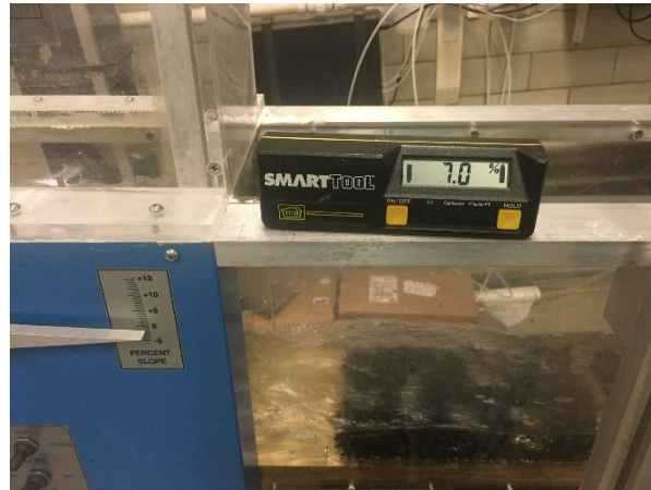
Figure 3.24 Slope measuring device
