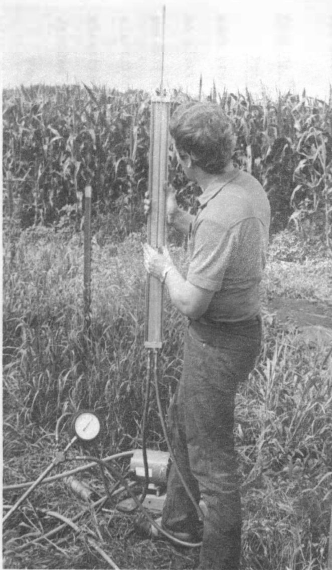
Figure 11. Measuring Discharge with the Hall Tube.
