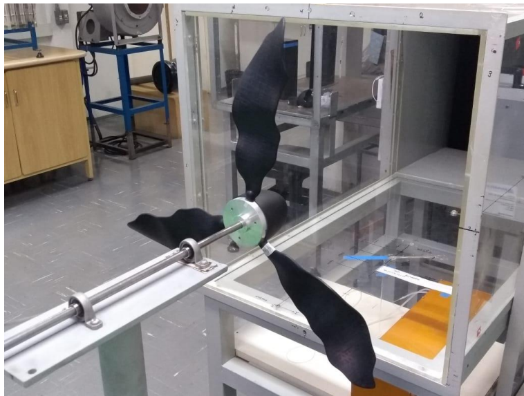
Figure 54. Bench for measuring performance of wind turbines at scale.
