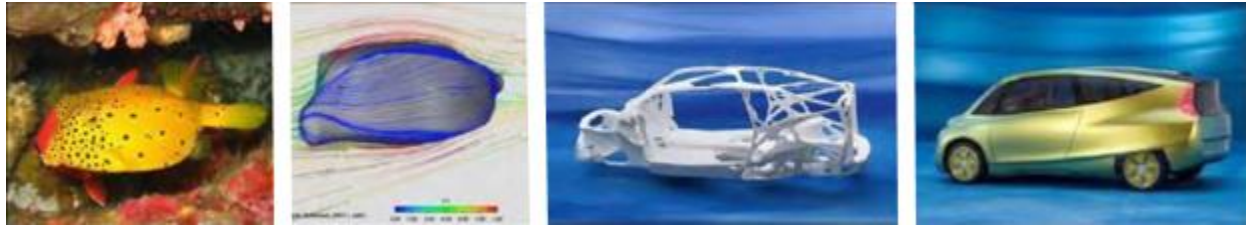
Figure 28. Daimle Chrysler bionic car inspired by the box fish and tree growth patterns.
