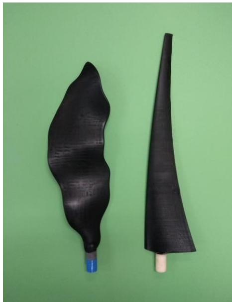
Figure 53. Final scaled model prototypes (reference and Q. Multiflora's blades).
