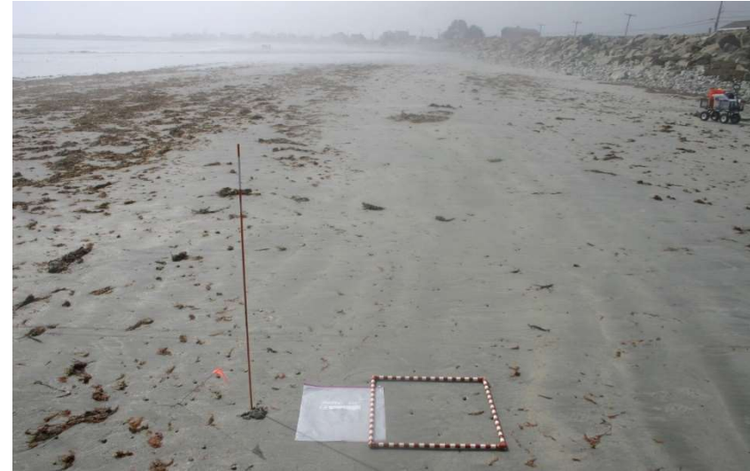
Figure FB-6. Foss Beach looking south from FB01 on April 9, 2017 (left photograph) after a period of erosion and on September 15, 2017 (right photograph) after a period of accretion. Note much of the lower gravel ramp exposed in April is buried by an accretional sand wedge in September.
