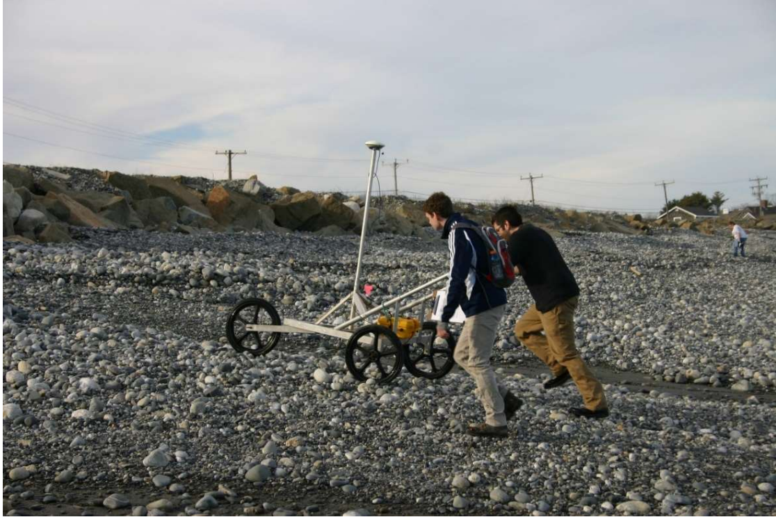
Figure 5-5. Running a beach elevation profile using the GNSS rover on the gravel ramp at Foss Beach station FB02 on April 9, 2017.
