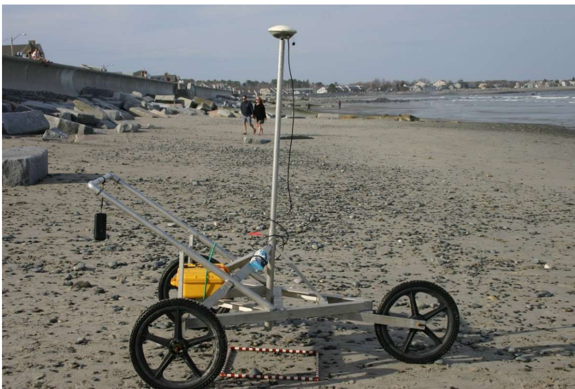
Figure 5-1. GNSS rover used to measure beach elevation profiles and locate sediment sampling stations. The photograph is looking north from station NB02 at North Beach on April 11, 2017.
