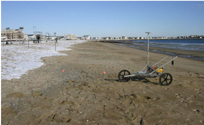
Figure HB-7. Station HB02 on February 3, 2017 looking north from the berm crest. The sediment sampling station is shown up close by the red flag in the lower photograph. The sediment was coarser overall in February than September at Hampton Beach. Very coarse sand to granule occurred on the berm crest.
