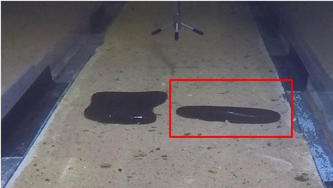
Figure 3-6: Rope formation (red box) at U=0.13 m/s during Trial 4 (FC oil, 25°C, sand).
