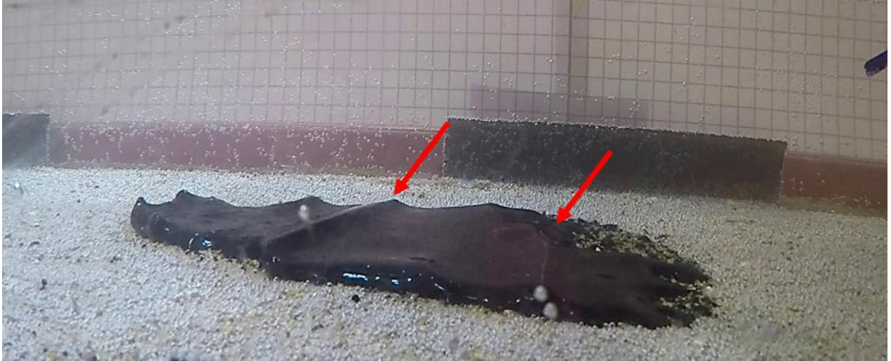
Figure 3-7: Ripple formation (red arrows) at U=0.27 m/s during Trial 8 (WC oil, 24°C, sand).
