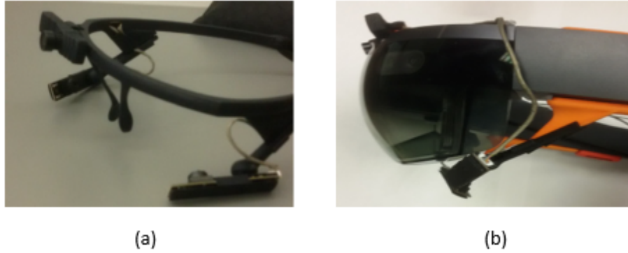
Figure 1.2. a) Pupil Lab's eye tracker. b) HoloLens with eye-tracker mounted on it
