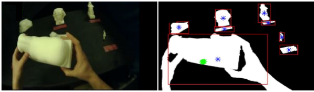
Figure 3: A frame from the eye tracker’s world camera with the artifact (white) and the description (red)(right). (b) The same image after being processed to identify the artifact and description AOI(left)
