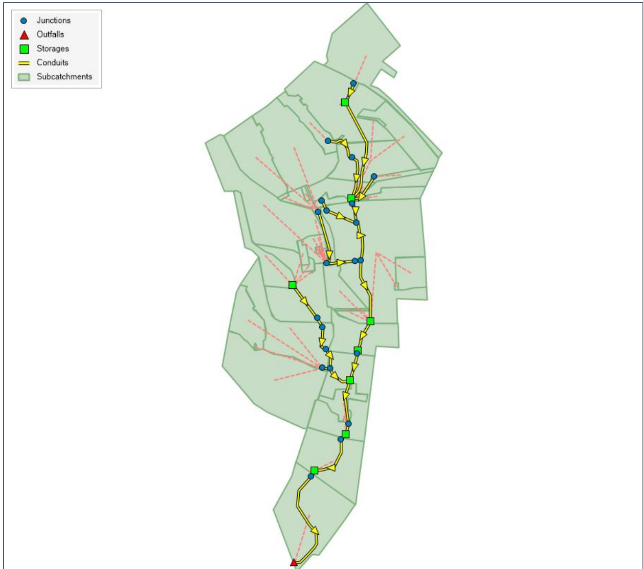
Figure 7: PCSMM Model of Pre-improvements Watershed. The dark green lines show subcatchment boundaries. The dotted red lines indicate to where subcatchments drained. Arrows indicate the direction of flow.
