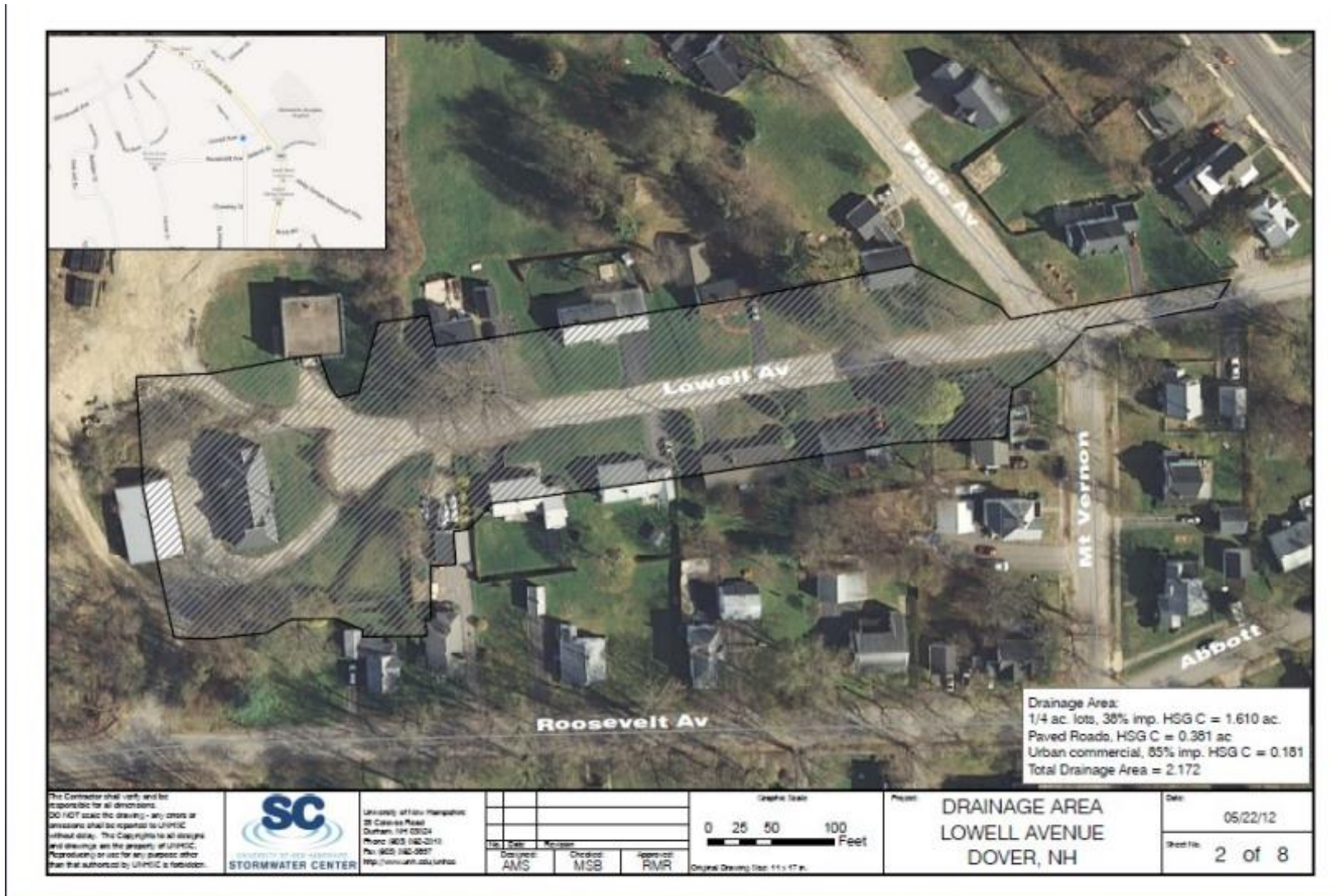
Figure 81: Lowell Avenue Bioretention drainage area
