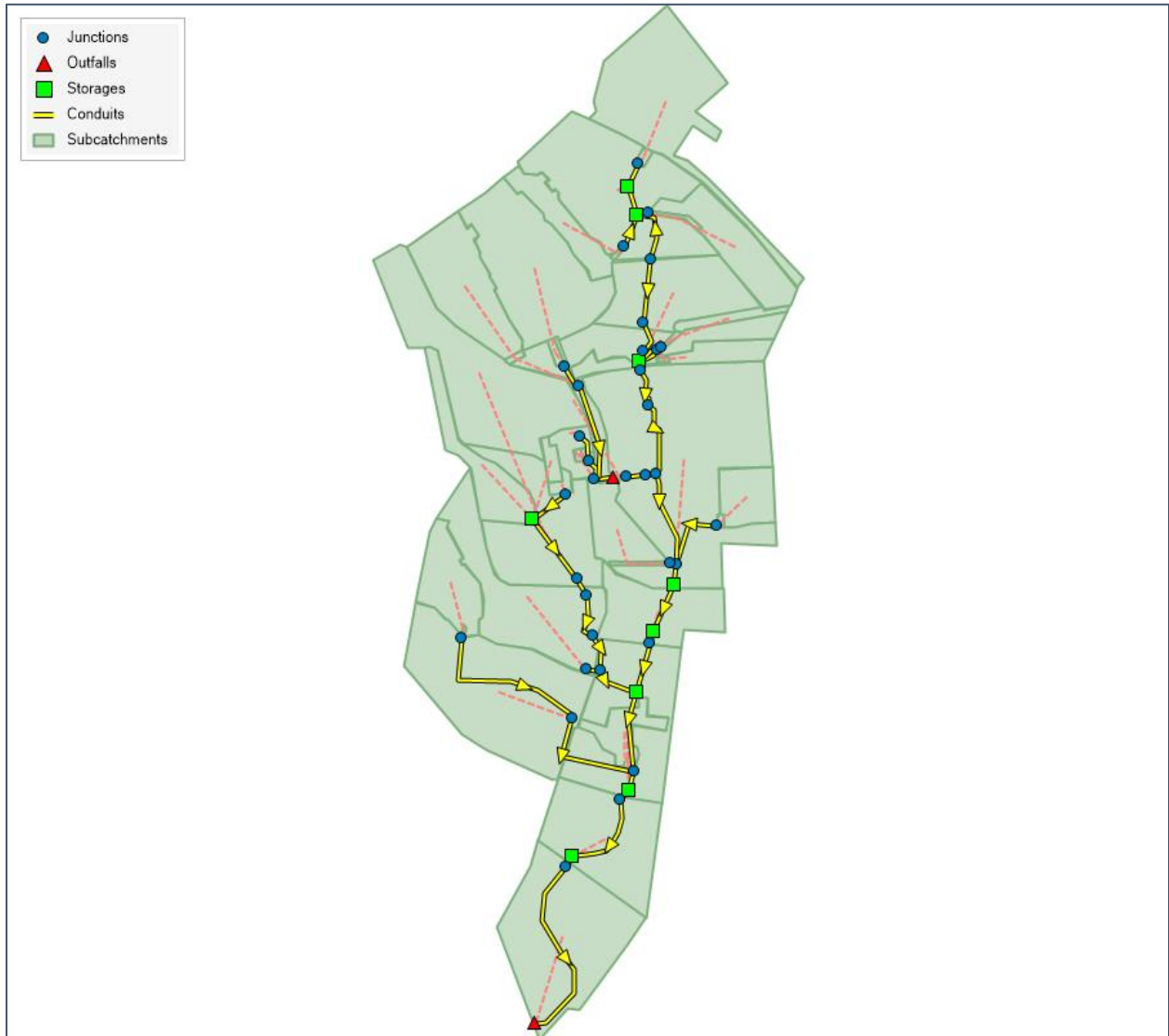
Figure 8: PCSWMM Model of Post-Improvements Watershed. The dark green lines show subcatchment boundaries. The dotted red lines indicate where subcatchments drained to. Arrows indicate the direction of flow.
