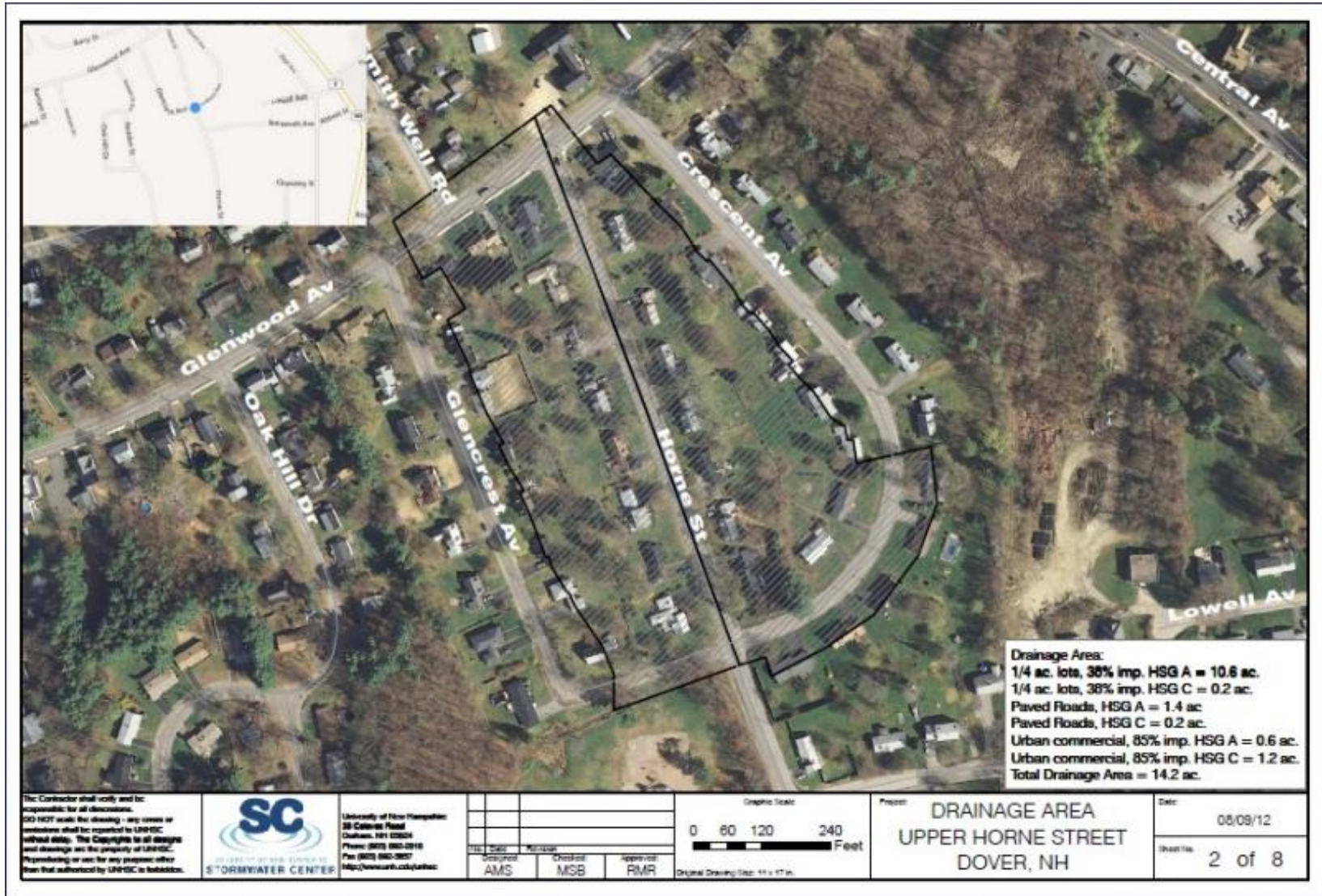
Figure 78: Upper Horne Street Bioretention drainage area
