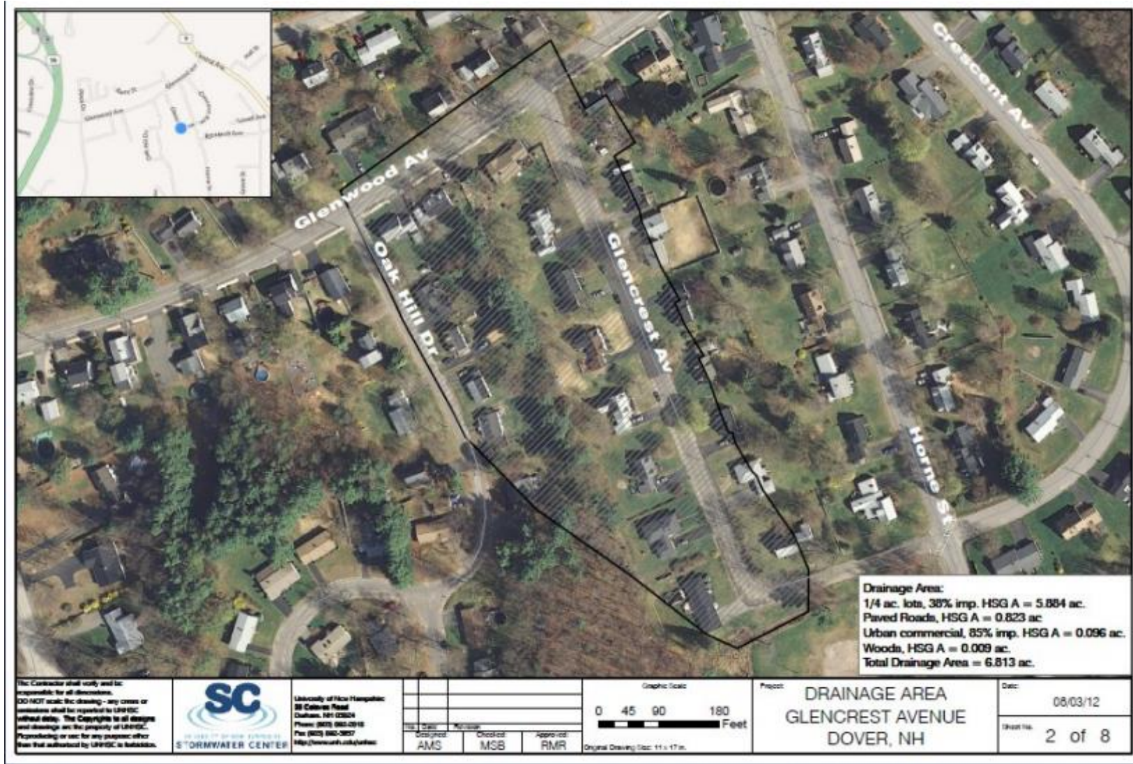
Figure 64: Glencrest Avenue Bioretention drainage area
