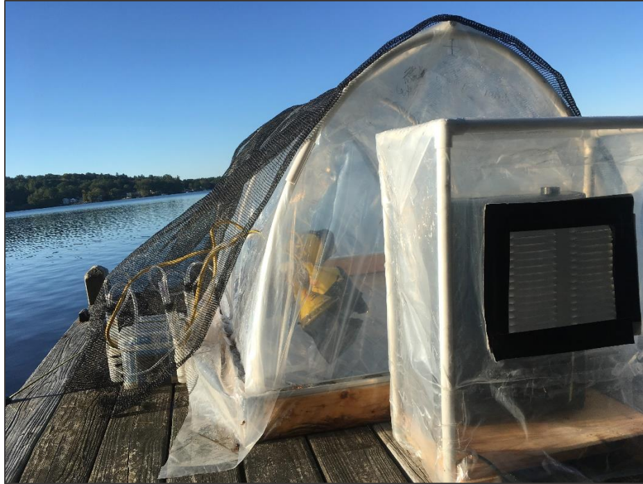
Figure 15. Placement of the CLAM unit to collect air from inside the HEPA filtered tunnel. The side of the tunnel was cut and re-sealed to allow the funnels to collect air from inside the tunnel, while the air pumps and traps remained outside on the dock.
