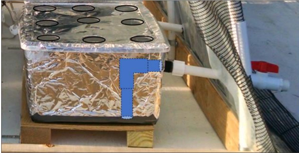
Figure 5. Individual hydroponic reservoir design constructed of a modified clear plastic storage bin. For each reservoir, nine holes were drilled in the lid to support nine plants, a small hole was drilled in the upper corner to allow for the aeration line, a plumbing system was constructed to drain and refill the reservoir, and foil was used to block out sunlight. Duct tape was used on the bottom edges to prevent the foil from tearing. Reservoirs were placed on individually leveled platforms to ensure water levels inside the reservoirs were uniform. Not pictured: Black plastic was later used to cover the lids to prevent seedlings from being burned by excess sunlight reflected off the foil
