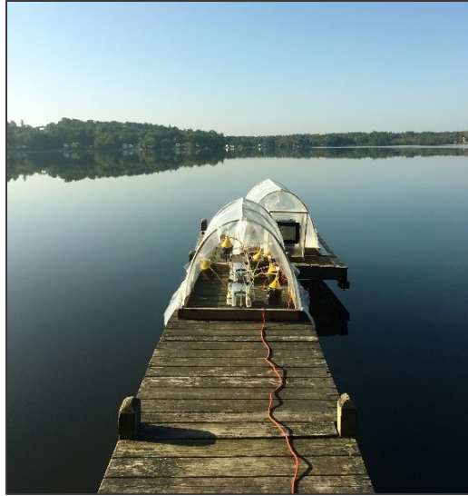
Figure 12. Two experimental tunnels with three CLAM units to measure lake aerosols inside the open-ended and HEPA filtered treatments during late September and early October of 2017.
