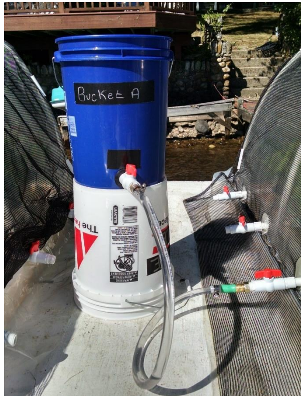
Figure 9. Refilling a reservoir with fertilized tap water using the modified 18.9 L (5 Gal) bucket.
