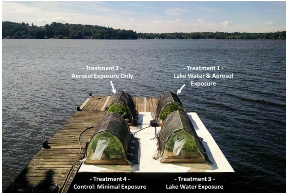
Figure 6. Four experimental treatment tunnels constructed on the dock expansion. Treatments 1 and 2 are open-ended to allow for free flow of air and exposure to cyanotoxin aerosols emitted from the lake. Treatments 3 and 4 are fully sealed and fitted with HEPA filters to remove particulate aerosols from the air entering these tunnels. In this image, the outflow ports for treatments 3 and 4 are visible; the HEPA filters are on the other side of the tunnels. Treatments 1 and 3 have lake water in the hydroponic reservoirs to expose plants to cyanotoxins directly via root uptake, where treatments 2 and 4 have tap water in the reservoirs to prevent this type of exposure. Shade-cloth was used to reduce temperatures inside the tunnels.
