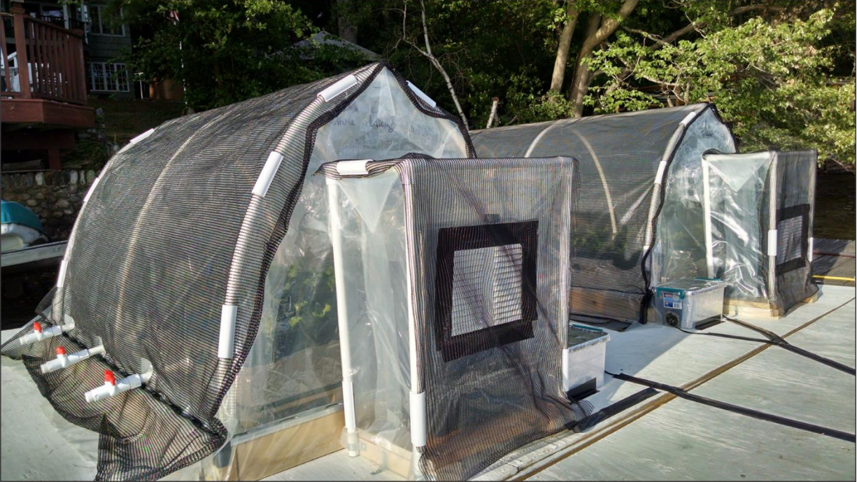
Figure 7. Image of Treatments 3 and 4 fitted with HEPA filters to exclude particulate aerosolized cyanotoxins. To protect the HEPA filters from rain, smaller enclosures were constructed out of PVC tubing, plywood, 2 x 4 ft boards, greenhouse film, and shade cloth. Home attic soffit vents were placed on one side to allow for inflow of air into the air filter, while preventing rainwater from entering. HEPA filters were placed inside the enclosures, which were connected to the treatment tunnels with greenhouse film. Also visible are the drain/fill pipes of three reservoirs as well as the boxes that were constructed to store the aeration pumps for each treatment tunnel.
