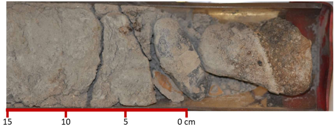
Figure 9. Photograph of the surface of vibracore UNH-1. Note lag deposit with cobble at surface of vibracore (above scale). Top of the core is to the right.
