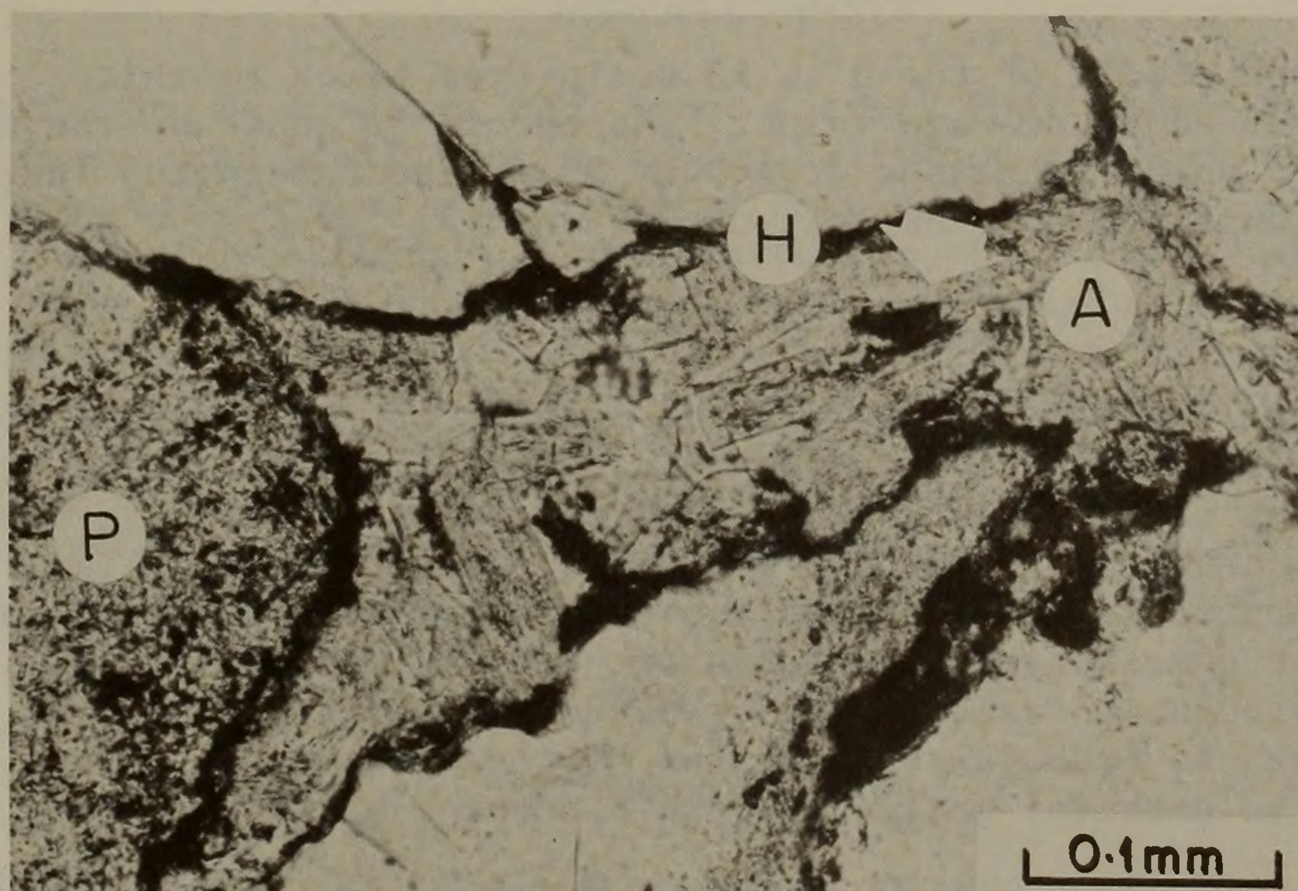
Fig. 19. Cement of albite (A), in part as crystals, fills former pore space in Buckland brownstone. The albite contains abundant dust inclusions. Hematite (H) stains occur on the detrital grains, including an altered plagioclase (P). "Late" authigenic hematite (arrow) stains some of the albite crystals.
