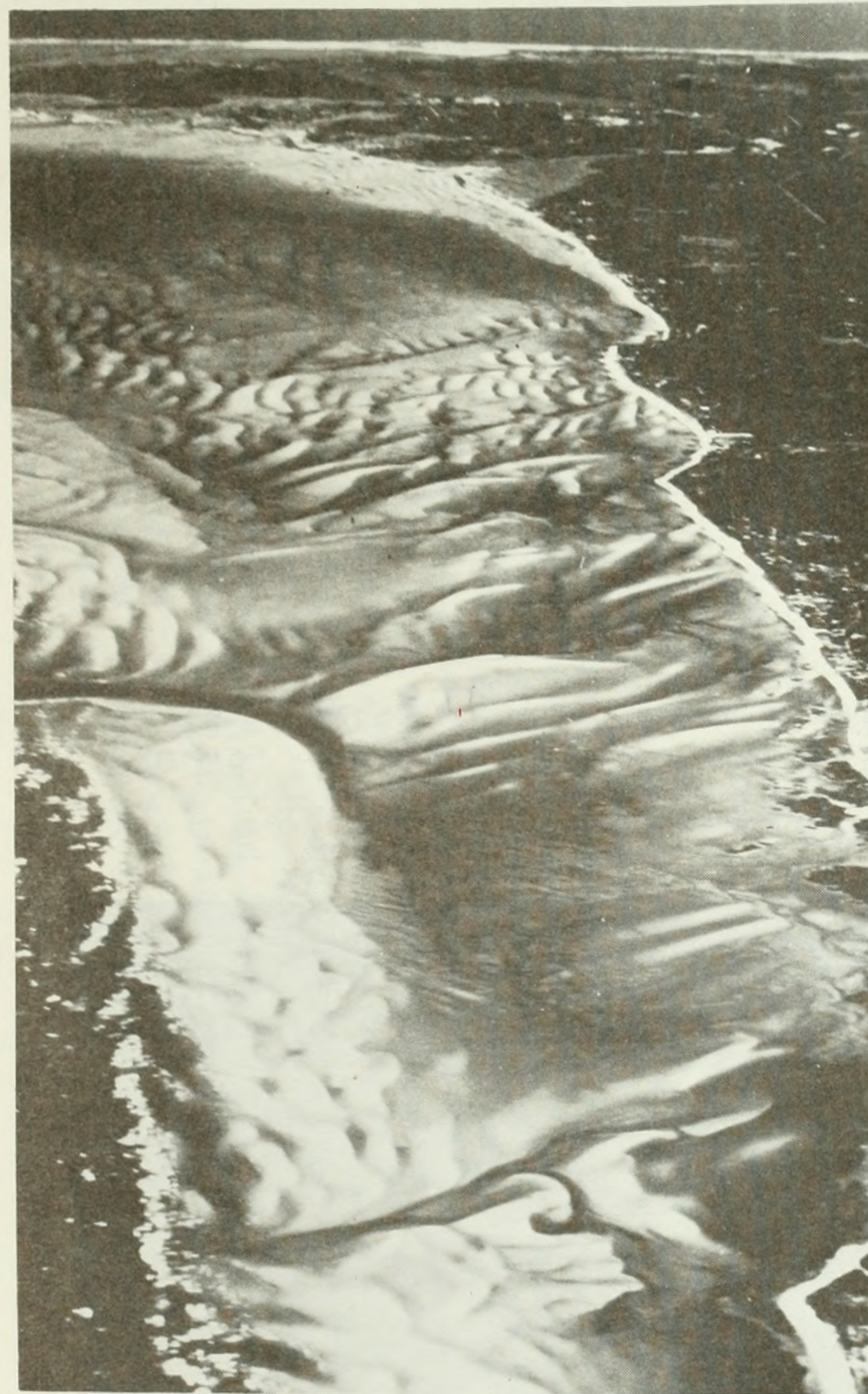
FIG. 4. Aerial Photo of the Brewster Tidal Flats Looking Eastward. Visible Features Include Crescent-Shaped Swash Bars, Curved Tidal Drainage Channels, Eastward Longshore Drift Shown by Sand Trapped by Grains.
