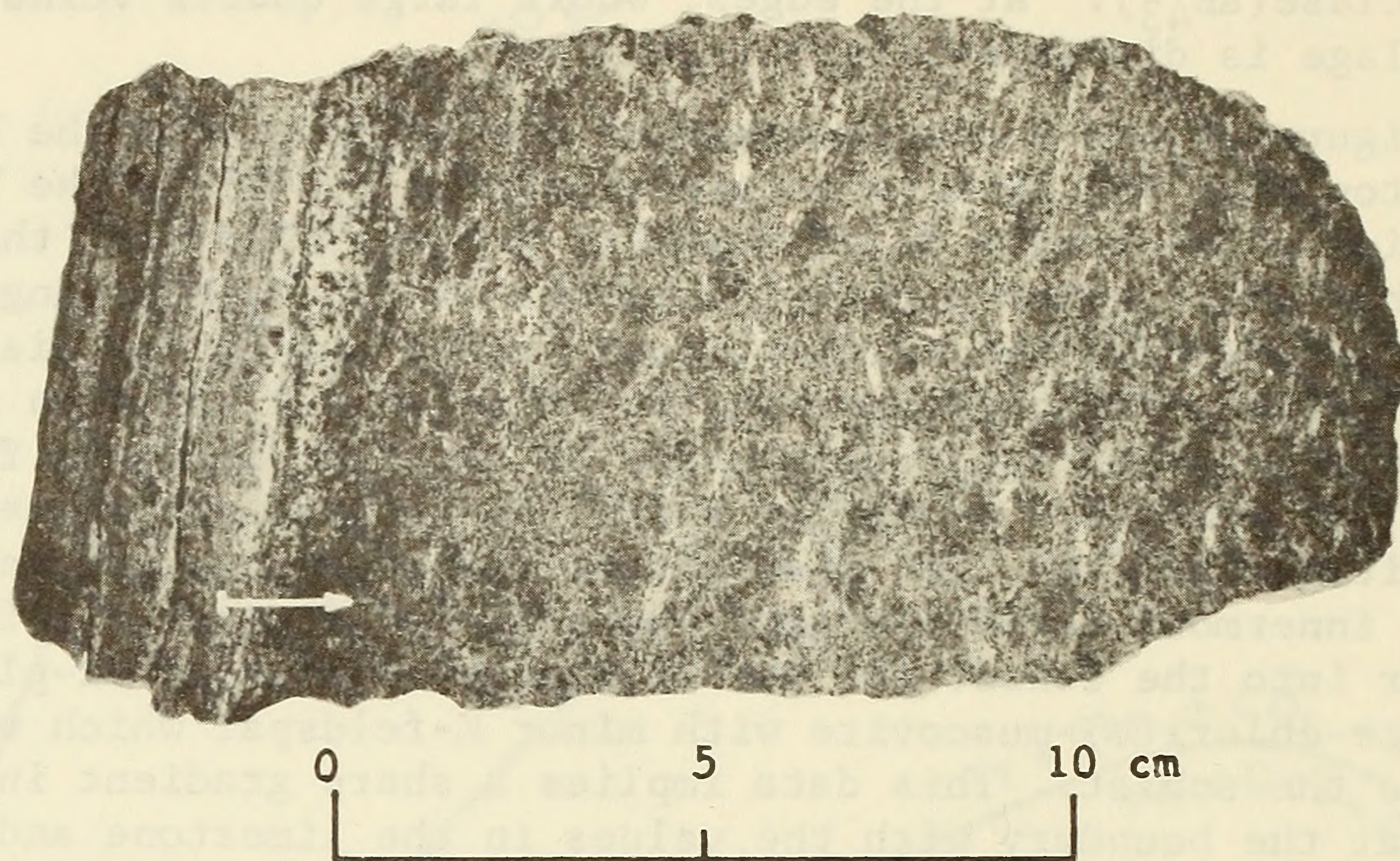
Fig. 4. Kyanite grade schist-micaceous limestone contact (Wep-16c). The arrow represents the path covered by the electron microprobe traverse.
