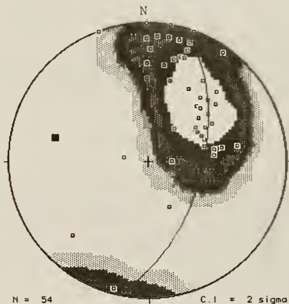
S1 foliation from the Lockwood Brook area Great circle based on F2 concentration; black square is fold axis, 32°, N76W
