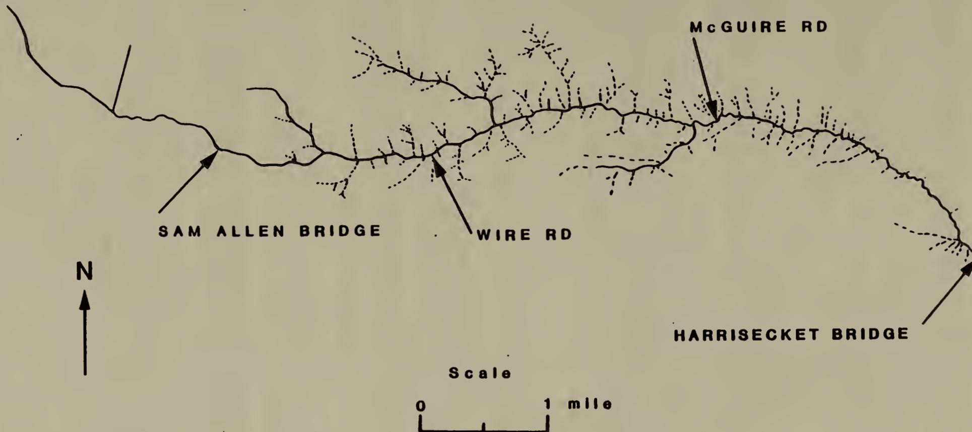
Figure 7. Pectinate drainage pattern of Branch Brook (dashed lines represent ephemeral streams). All of the larger tributaries have become reoriented in the direction of maximum or preferred hydraulic conductivity which is in the flow direction of the glacio-fluvial meltwater streams of the retreating Wisconsin Ice Sheet.
