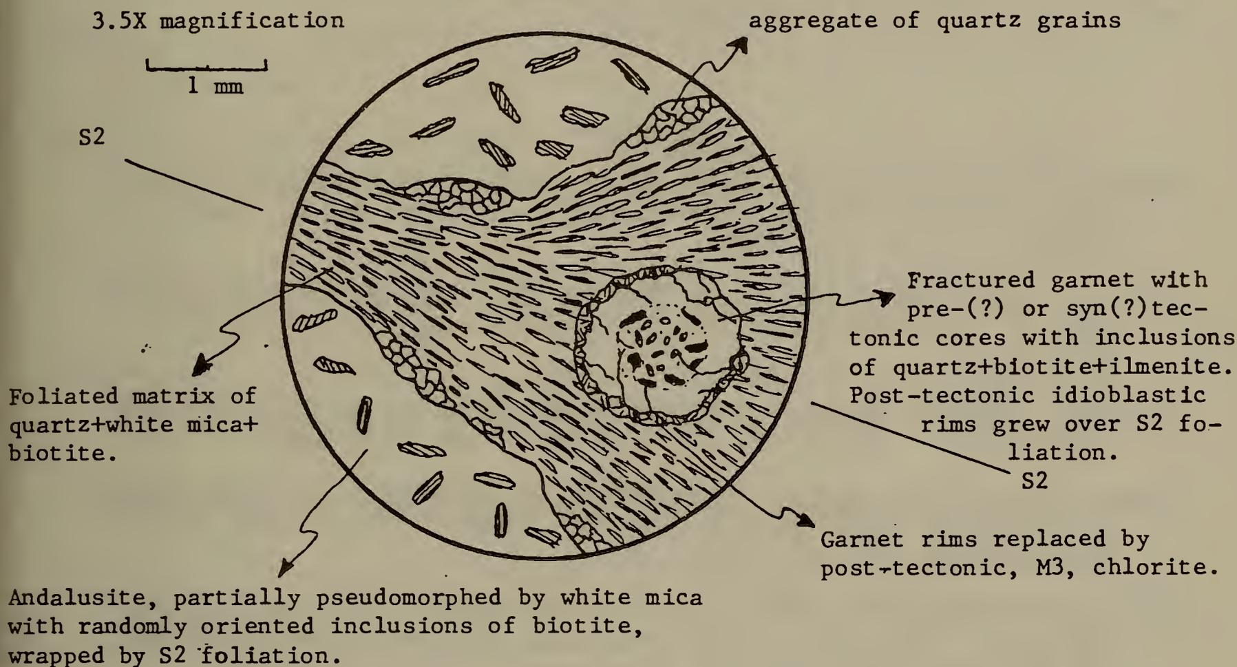
FIGURE 7 Textural sketch of thin section from Unit 4. Sample from East Rochester about .5 mile downstream along the Salmon Falls river from STOP 4.
