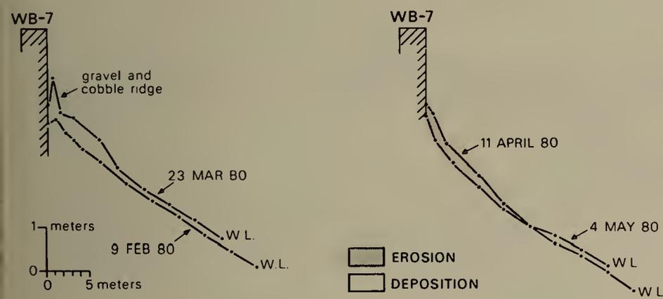
Figure 37. Profile changes to the beach. Note deposition that occurred after the initial riprap was placed along the seawall and the subsequent storm induced erosion. Some of the eroded gravel transported over the seawall.
