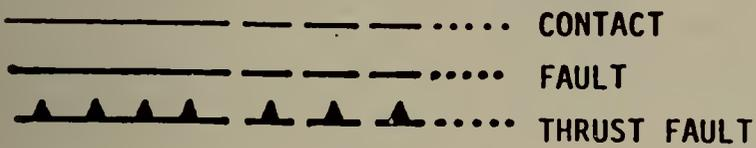
Contacts and faults drawn where approximately located, dashed where inferred and dotted where probable. Direction of movement along the faults was not be interpreted from field data.
