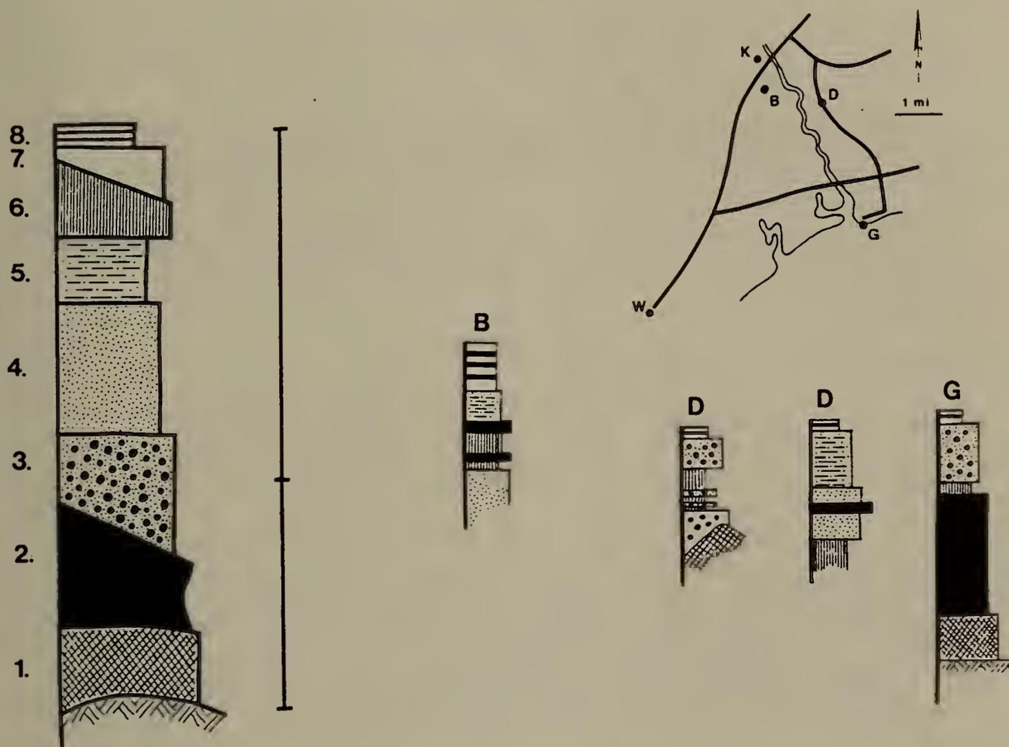
Figure 5. Summary of stratigraphy seen at Stops 1, 1a, 2, and 2a. Explanation: K - Kennebunk, B - Brown's Road, D - Kennebunk landfill, G - Great Hill, W - Wells. 1 - Massive diamicton, 2 - Bedded diamicton, 3 - Poorly-sorted and stratified gravel, 4 - Sorted and stratified sand and gravel, 5 - Laminated silt and sand, 6 - Massive/laminated silt and clay, 7 - Organic mud, 8 - Well-sorted stratified sand.
