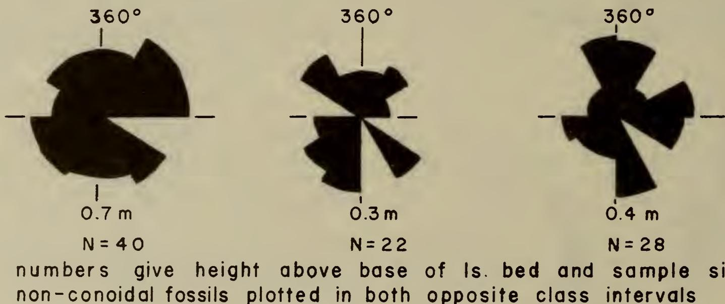
Figure 5. Circular histograms (equal area) showing orientations of long axes of hyoliths measured in slabs and peels parallel to bedding.
