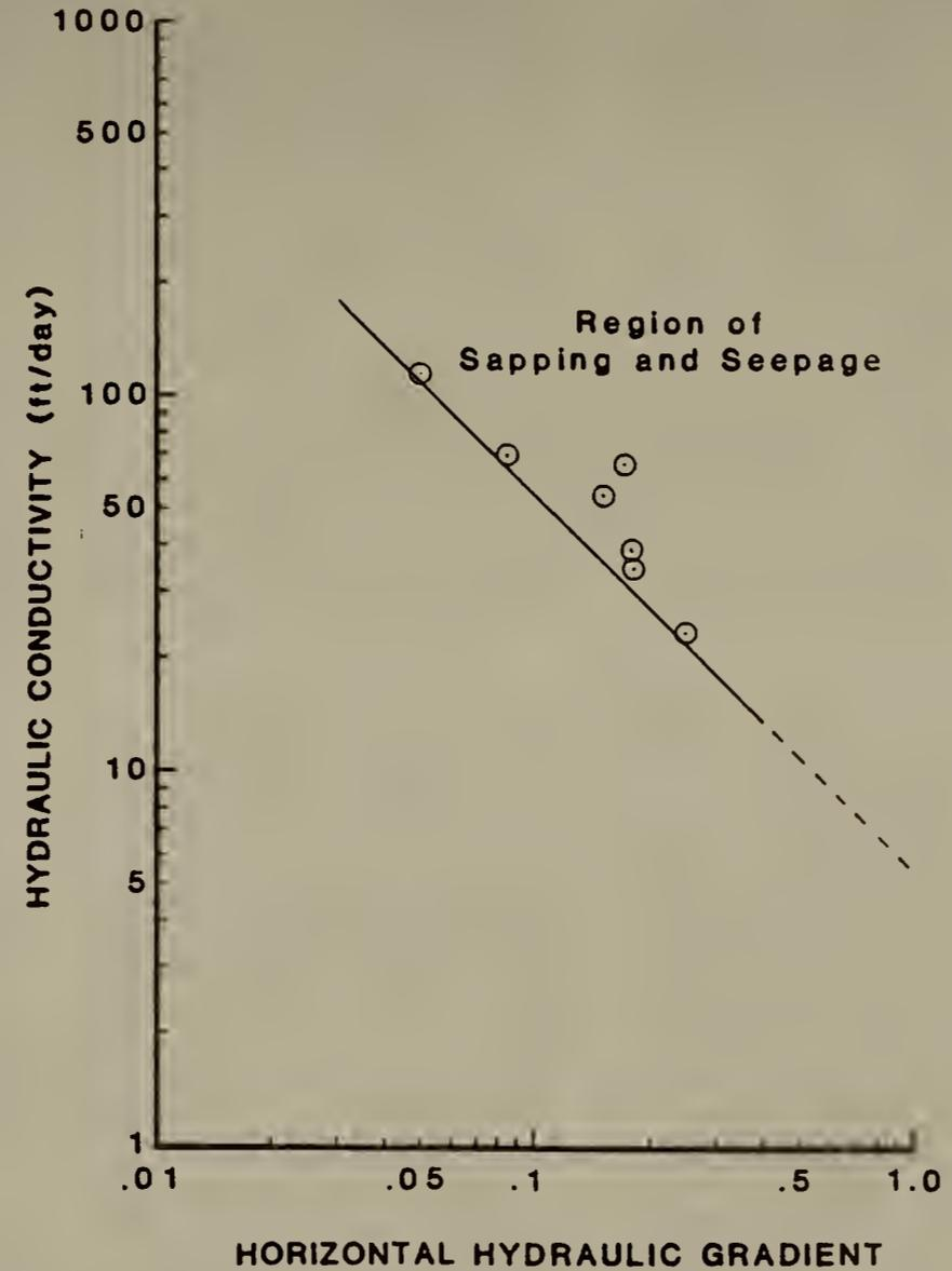
Figure 6. Relationship between hydraulic conductivity and horizontal hydraulic gradient. The solid line represents a theoretical approximation of the minimum slope necessary for the initiation of sapping and seepage in unconsolidated sediments of similar densities. The circles are measured values.
