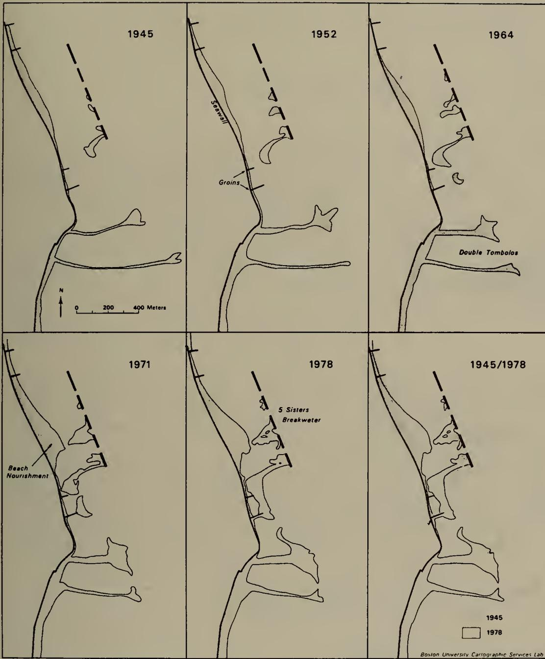
Figure 25. Historical morphological changes of the double tombolo system and gravel bars at the Five Sisters Breakwater.
