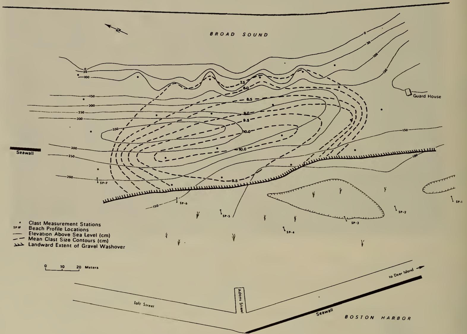
Figure 13. Topographic map and grain size distribution of gravel washover. Note that clast size increases in a landward direction.
