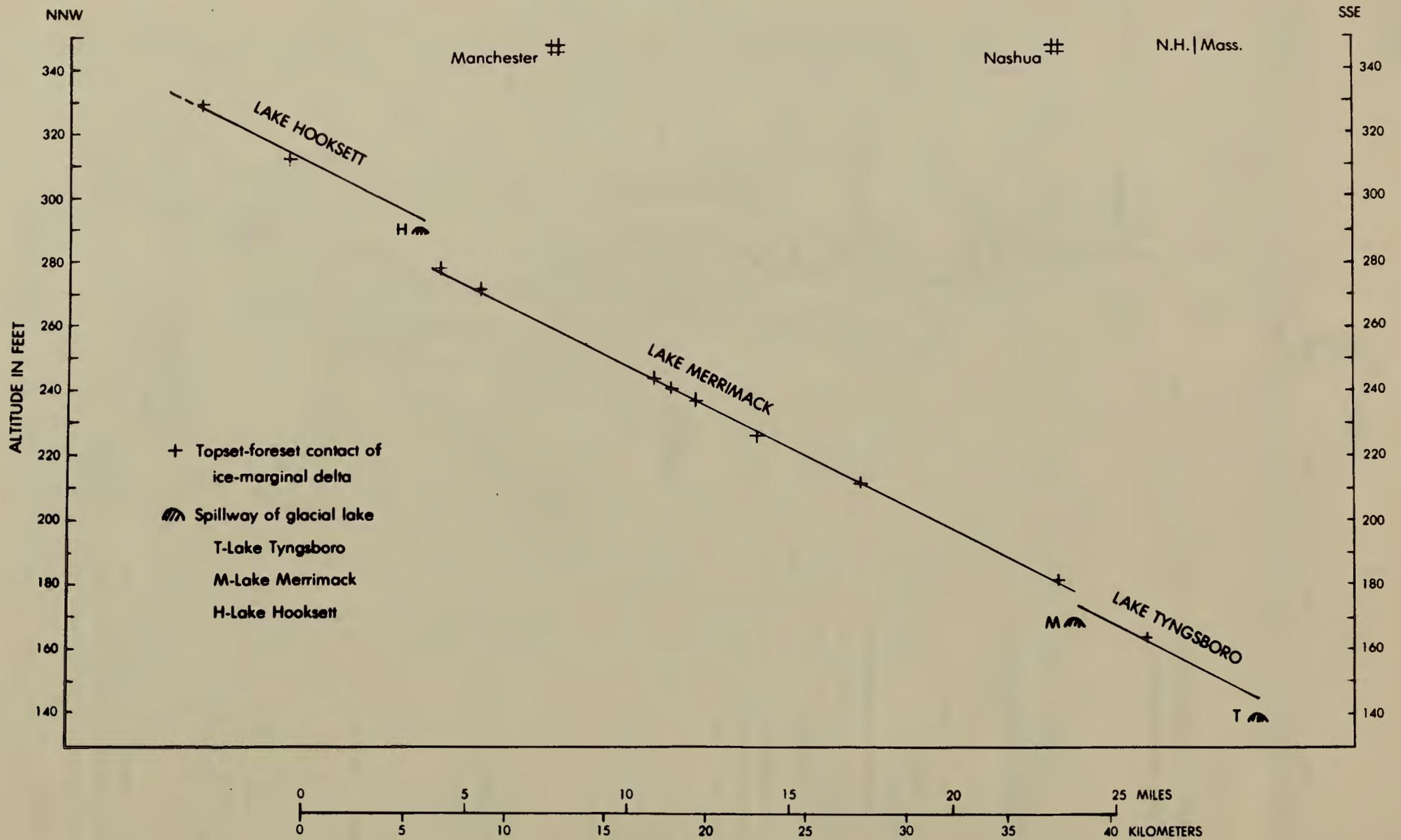
Figure 2. Profiles of glacial-lake levels in the Merrimack Valley. Projected gradient is 4.7-4.9 ft/mi (0.89-0.93 m/km) up to NNW. Direction based on best fit by inspection of line to the data points.
