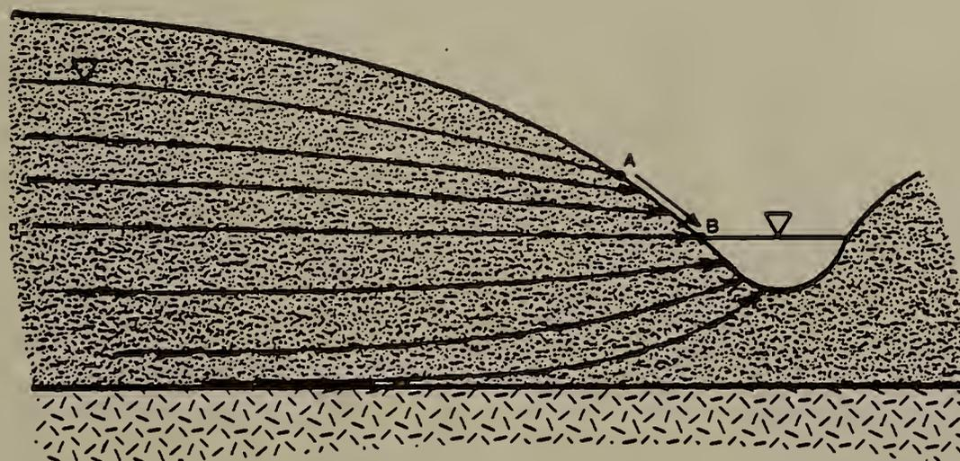
Figure 3. Groundwater discharge along a seepage face. Whenever a phreatic surface approaches a downstream external boundary of a flow domain, it will always terminate on it at a point (A) that is above the water table. The surface A B represents the seepage face (after Bear, 1979).
