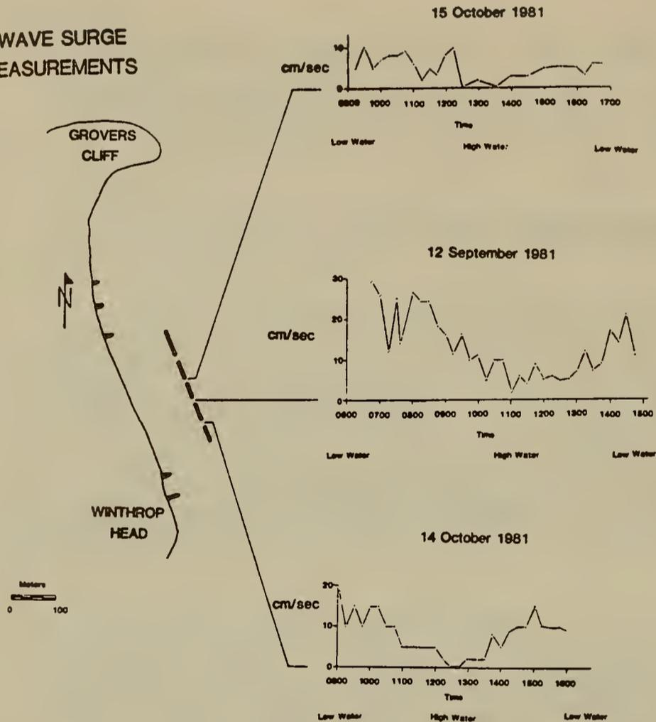
Figure 29. Wave surge current velocities measure between the sections of the Five Sisters Breakwater (from Sullivan, 1981).
