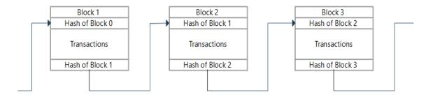
Figure 2.2: Structure of Blockchain
