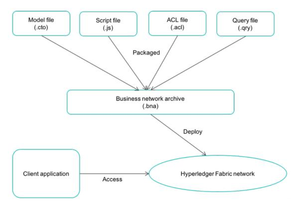
Figure 3.2: Components of Blockchain [54]
