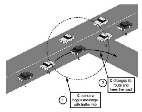
Figure 1.2: Example of an attack [8]
