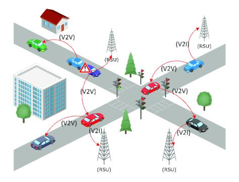
Figure 2.1: V2V and V2I communication [13]
