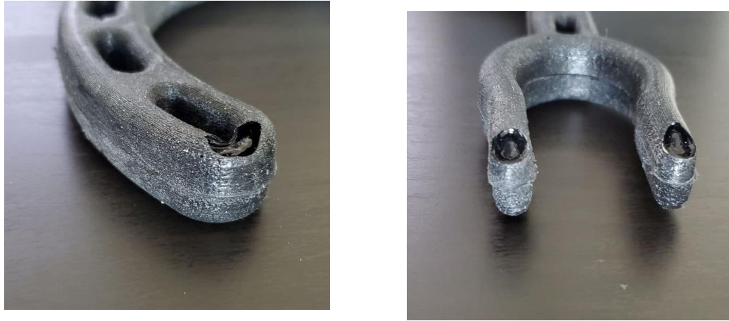
Figure 4.10 Formation of air bubbles at both ends of J-hook
