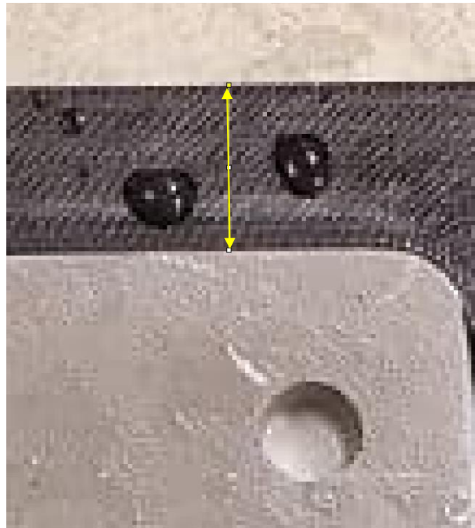
Figure 4.21 Setting a measurement scale for the flash calculation
