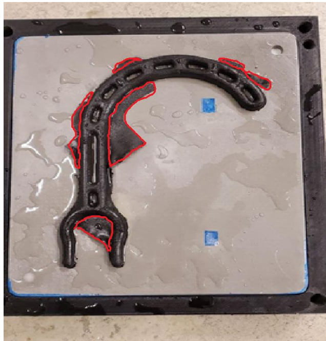
Figure 4.7 The injected J-hook right after opening the mold package (Red areas show the excess material “flash” that is inevitable an injection molding process)
