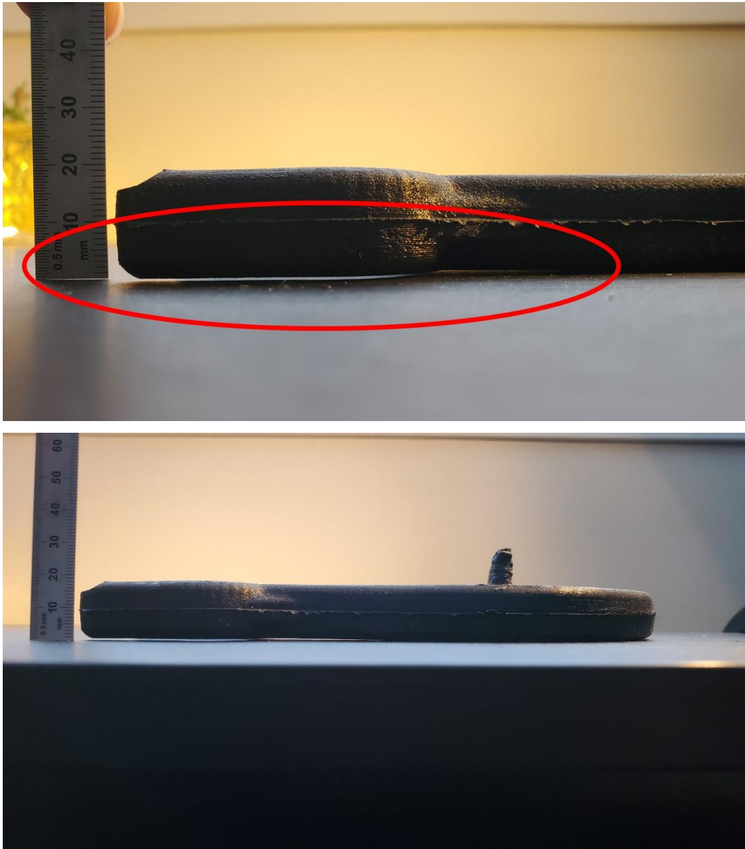
Figure 4.12 Measuring the flatness of the J-hook
