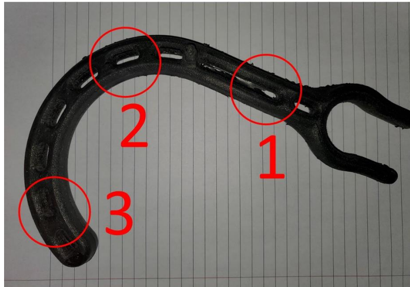
Figure 4.13 Selected areas for dimensional measurements
