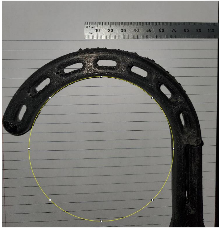
Figure 4.18 The circle fitted to the inside arc by ImageJ software
