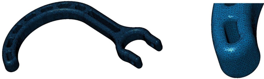
Figure 3.8 The discretized mesh and the magnified view of the version 2 FEA model
