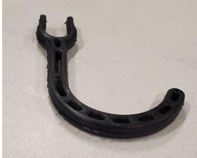
Figure 4.8 Final J-hook after removal of the flash
