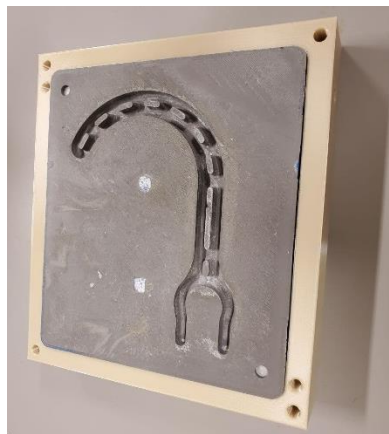
Figure 4.4 Cured epoxy (top); After dissolving the patterns (middle); And final assembled into mold box (bottom)
