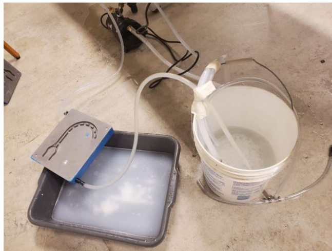
Figure 4.6 Testing the fluid flow and connecting the mold to the fluid circuit
