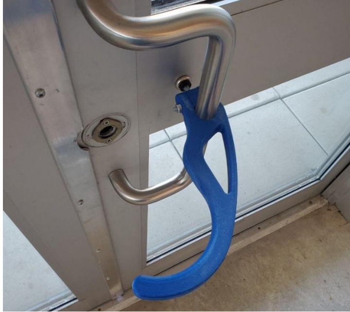
Figure 1.8 Extended door handle design built via FDM technology. Material price for this handle cost around 50 CAD
