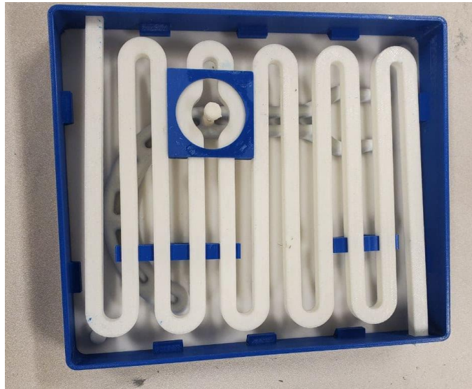
Figure 3.25 Configuration of the top cavity prior to casting epoxy
