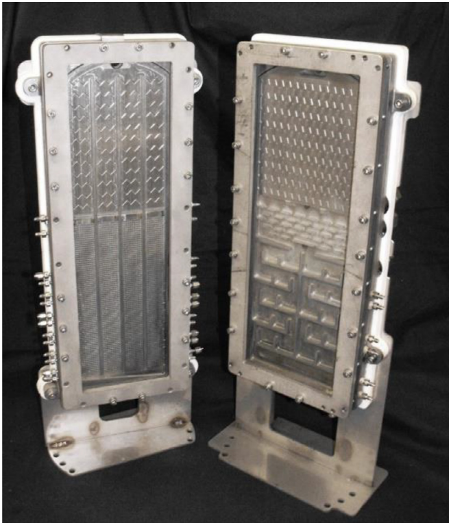
Fig. 12. Vertical column (left) and branched tray (right) test sections [98].
