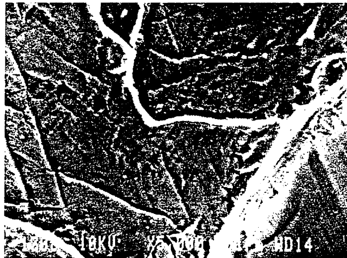
Figure 3.16 Transgranular fracture in \delta -ferrite in the hydrogen-induced cracking zone, from the same specimen as Fig. 3.15.
