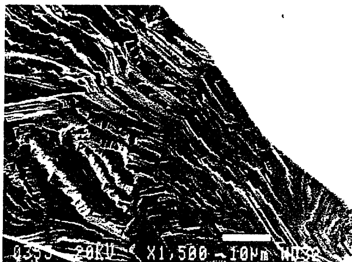
Figure 6.8 Relatively low K features of transgranular SCC fracture in annealed CT specimens.
