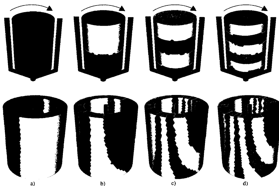
Figure 6-14. Partitions used to test the parallel performance of an agitated tank with baffles simulation; a) 3 subdomains b) 6 subdomains c) 12 subdomains d) 16 subdomains.
