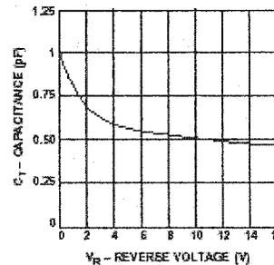
Figure 15. Total Capacitance vs. Reverse Voltage—HSMS-2810 Series.
