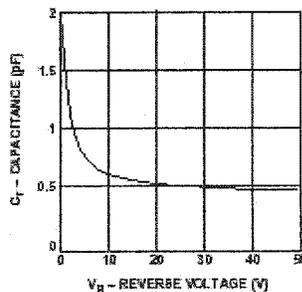
Figure 14. Total Capacitance vs. Reverse Voltage—HSMS-2800 Series.
