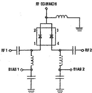
Figure 6. Simple SPDT Switch Using Only Positive Bias.
