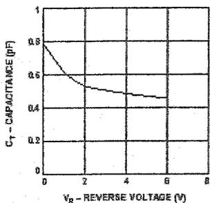
Figure 16. Total Capacitance vs. Reverse Voltage—HSMS-2820 Series.
