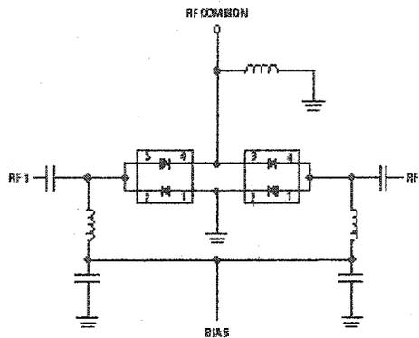
Figure 7. High Isolation SPDT Switch Using Dual Bias.
