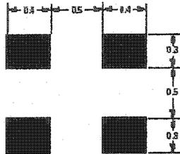
Figure 12. PCB Pad Layout, MiniPak (dimensions in mm).
