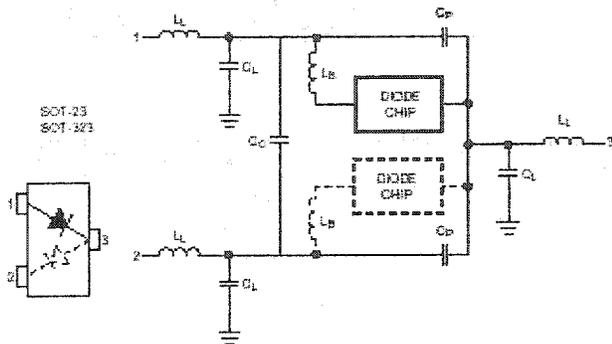
Figure 2. Model of the SOT-23 and SOT-323 packages
