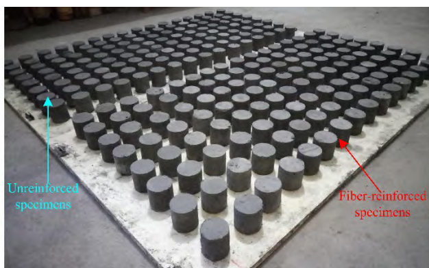
FIGURE 3. CPB specimens: fiber-reinforced and unreinforced.
