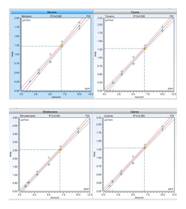
Figure 6. Calibration equation plots for benzene, toluene, ethylbenzene, and xylenes are given with confidence limits in red ( $\alpha$ =0.005). Yellow points indicate data point for selected injection and dotted lines indicate area and amount for selected data point.
