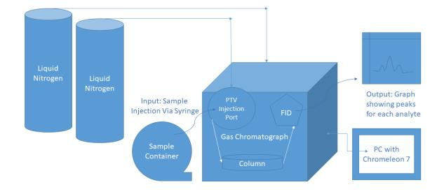
Figure 5. Diagram of current equipment setup and flow of sample analysis using GC-FID.
