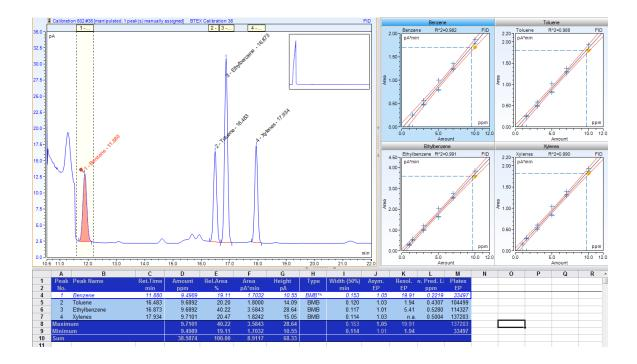
Figure 4. Representative chromatogram shows peaks for benzene, toluene, ethylbenzene, and xylenes analyzed during the calibration process. Each analyte had a retention window identified at the top of the chromatogram. Detector response was given on the y-axis in pA. Retention time was given on the x-axis in minutes.
