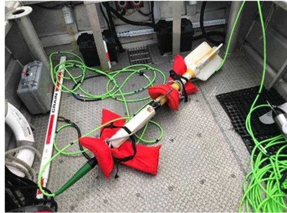
Figure 4-7. Geometrics G-882 Marine Magnetometer with life preservers attached for towing in shallow water.
