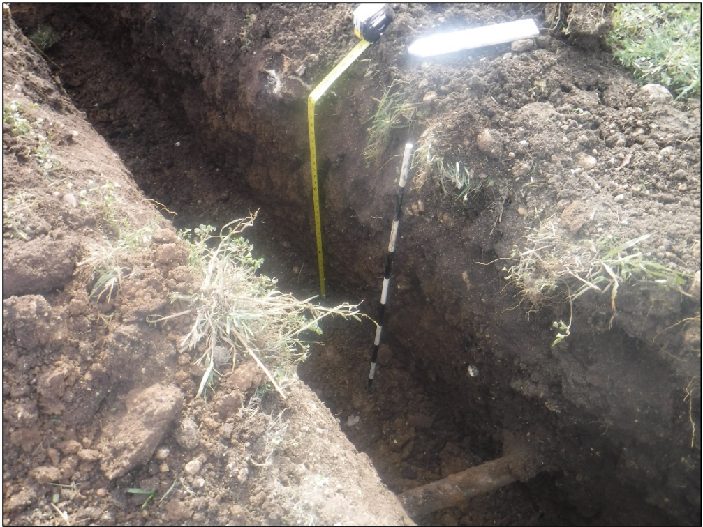
Figure 5-9. Average soil profile of the western APE excavation, showing existing utility line, facing east.
