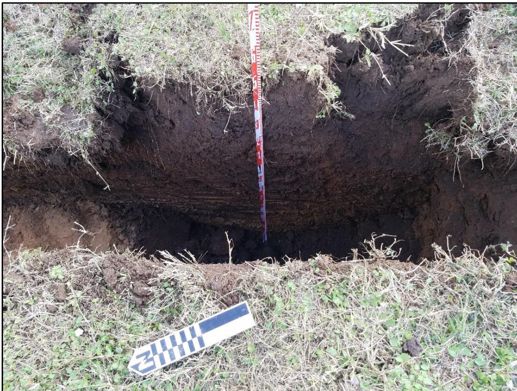
Figure 5-3. Average soil profile for intact soil deposits along the southwestern side of Martinez Losoya Road ROW.
