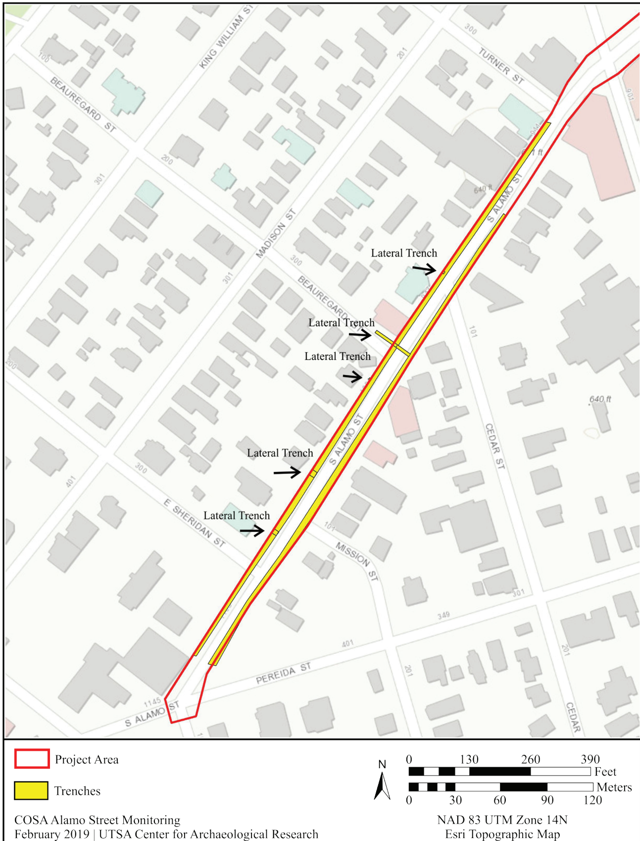
Figure 4-1. Trench locations within the project area.
