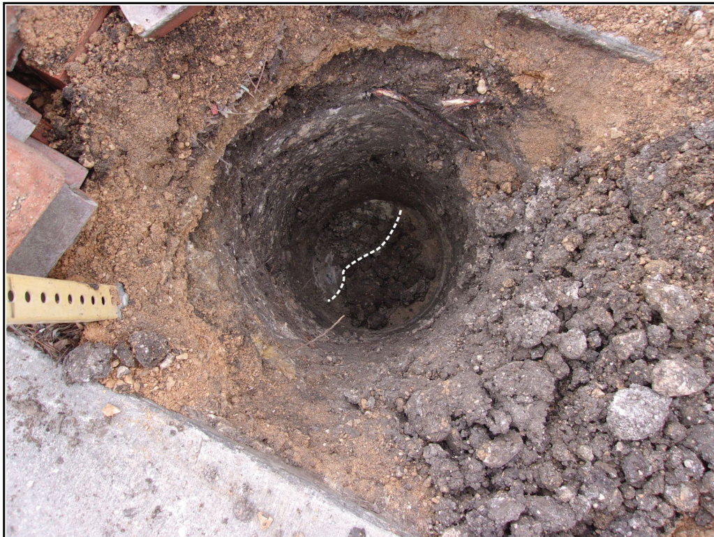
Figure 4-10. Borehole near acequia. Limestone obstruction at the bottom marked in white. Feature extends into the north (upper left) portion of the borehole wall.
