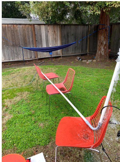
Figure 5.8: Flow loss test with long radius elbow
