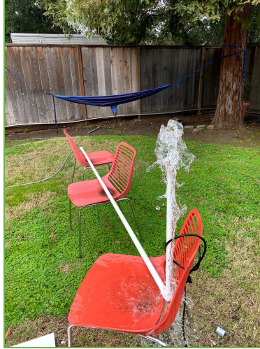
Figure 5.7: Flow loss test with short radius elbow
