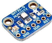
Figure 5.12: Adafruit Sensirion SHT31-D Temperature and Humidity Sensor ( reproduced without permission ) [17]
