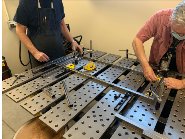
Figure 4.4: GRVLR Metal Frame Welding.
