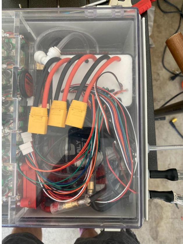
Figure 29: Unwired Motor Controller with Water Cooling Enclosure
