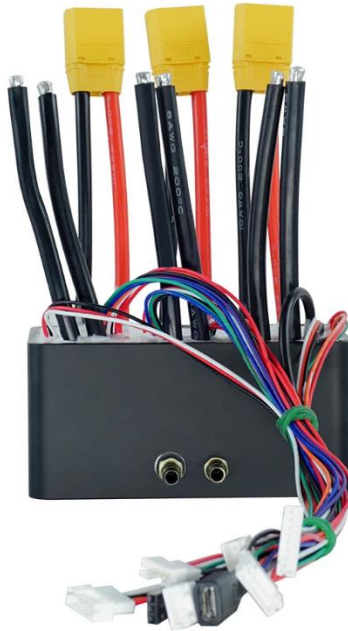
Figure 30: Flipsky FSESC 75200 75V High Current 200A ESC “Used Without Permission”
