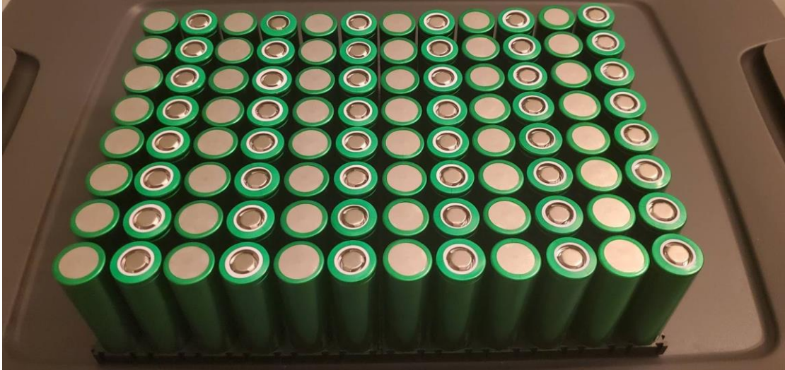
Figure 21: 18650 Lithium-ion Battery Cell Assembly
