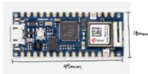
Figure 3.2: The Arduino Nano 33 IOT, which helps to remotely control the swimmer
