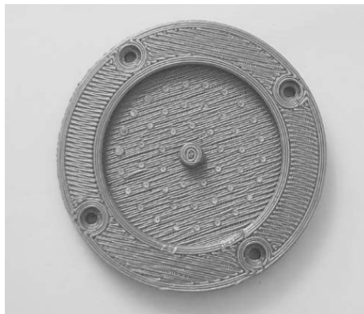
Figure 5.4: 3D printer swimmer lid
