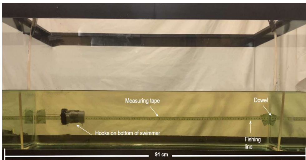
Figure 6.1: Swimmer inside the test ready tank
