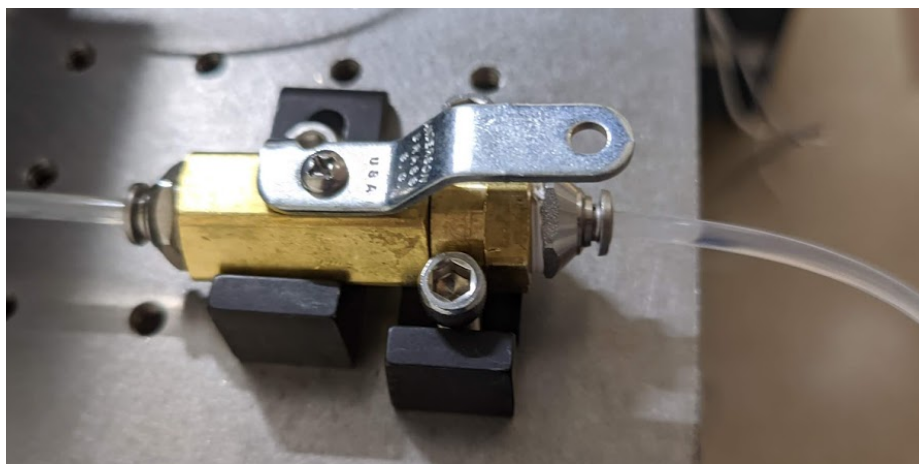
Figure 6.7: Flow regulator which controls the flow to the heat sink.
