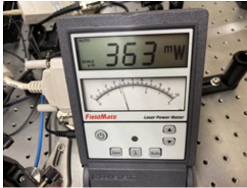
Figure 8.2: Power meter and sample reading.
