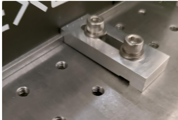
Figure 4.6: Steel clamps which clamp to the breadboard. Detailed engineering drawings of the breadboard clamps are included in Appendix C.4.
