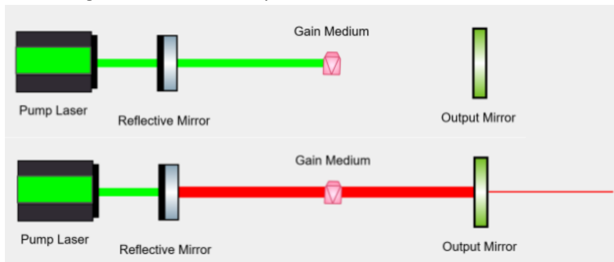
Figure 1.5: Two mirror optical resonator which supports lasing. The green beam is turned to infrared when it contacts the gain medium. The gain medium sends infrared light to the output mirror as well as back to the reflective mirror.
