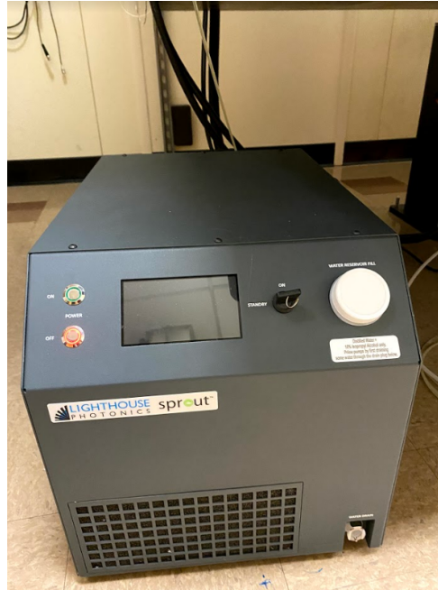
Figure 6.8: Sprout G pump laser power supply and liquid cooling pump (chiller).
