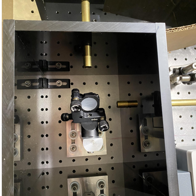
Figure 3.11: Top view of the periscope containment (shielding) box, with lid removed. The light-tight box was made using cellcast opaque acrylic and acrylic cement.
