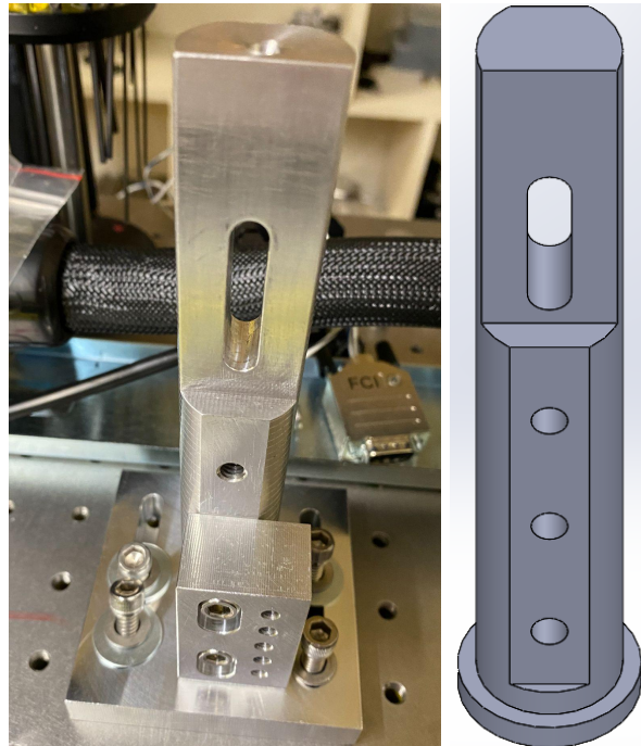
Figure 3.8: Left: Machined 6061 Al periscope tower, mounting plate and variable mirror mount. Right: The 6" tall x 1" diameter design model of the periscope tower.
