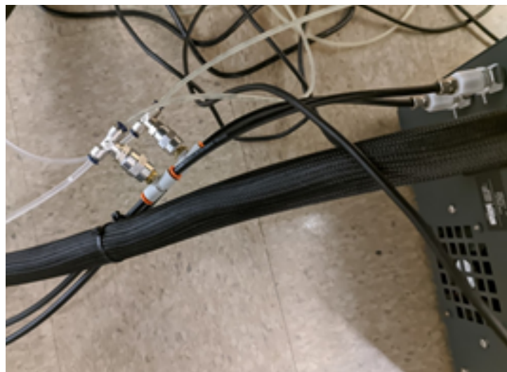
Figure 6.9: Junction for fluid pump that directs 0.17 L/min of cooling fluid to the OFHC heatsink of our Ti:Sapphire laser crystal.
