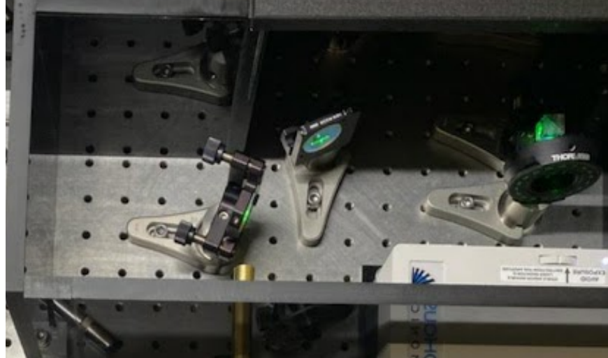
Figure 3.5: Mirror configuration in the original pump beam containment box.
