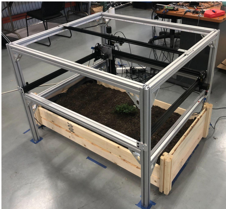
Figure 3.12: Final Cartesian Subsystem
