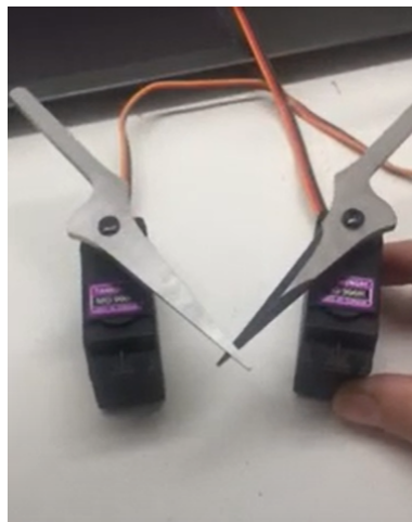
Figure 4.3: Preliminary Snipping Design
