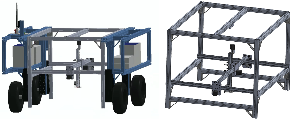
Figure 2.4 : Mechanical configuration of RoboCrop and Ag Robot II.
