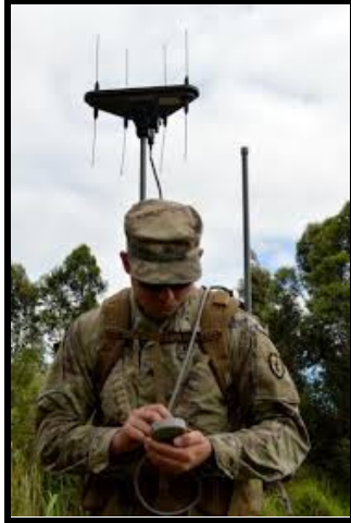
Figure 3: Wolfhound RF DF system used by United States Military for tactical RF DF operations [5]
